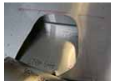
Start by making a small V cut in the trailing edge; cut through both the top and bottom side of the skin. Insert the snips between the skins, cut one side at a time.
