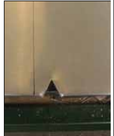
With the snips, start cutting in the middle of trailing edge.
