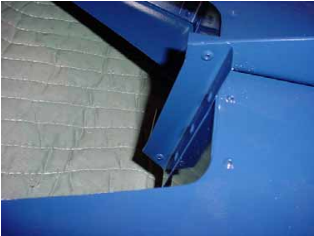
L Angle riveted to Channel 8H2-14
