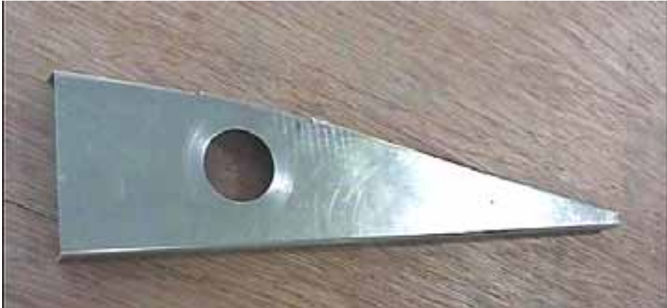
Tip rib with hole opened to 35 to 50mm to provide clearance for the elevator hinge ping and cotter pin.
