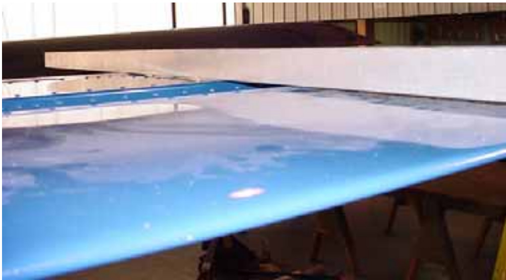
Elevator neutral position: lay a straight edge over the top of the stabilizer, bring the elevator to the straight edge.
