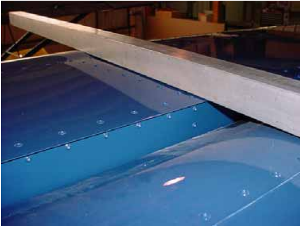
Straight edge on top of stabilizer to locate elevator neutral position
