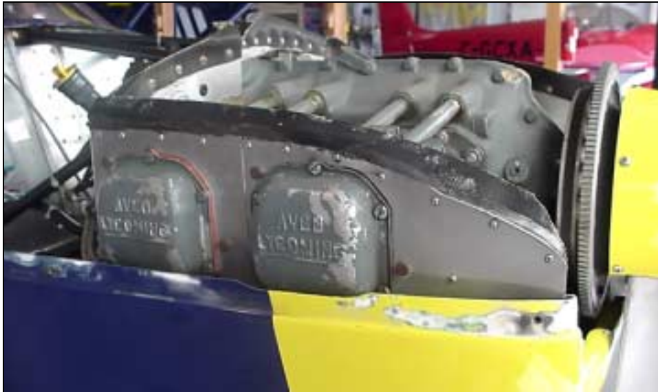
The right side baffles with the lower cowl installed.
