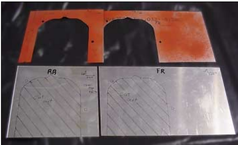
The right side baffles. Front (FR) and Rear (RR)
