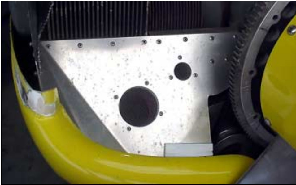
The installed right front baffle with the lower engine cowl.
