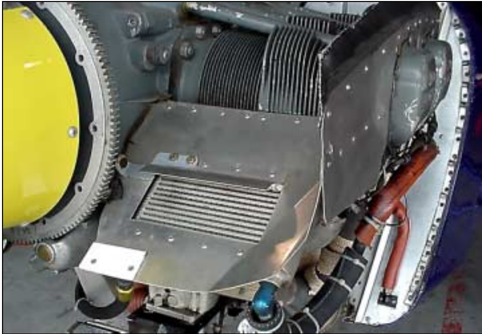
The left front baffle.
