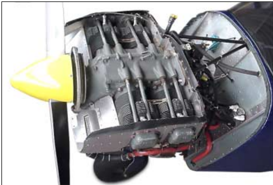
STOL CH 801 Lycoming O-360 engine with baffles
