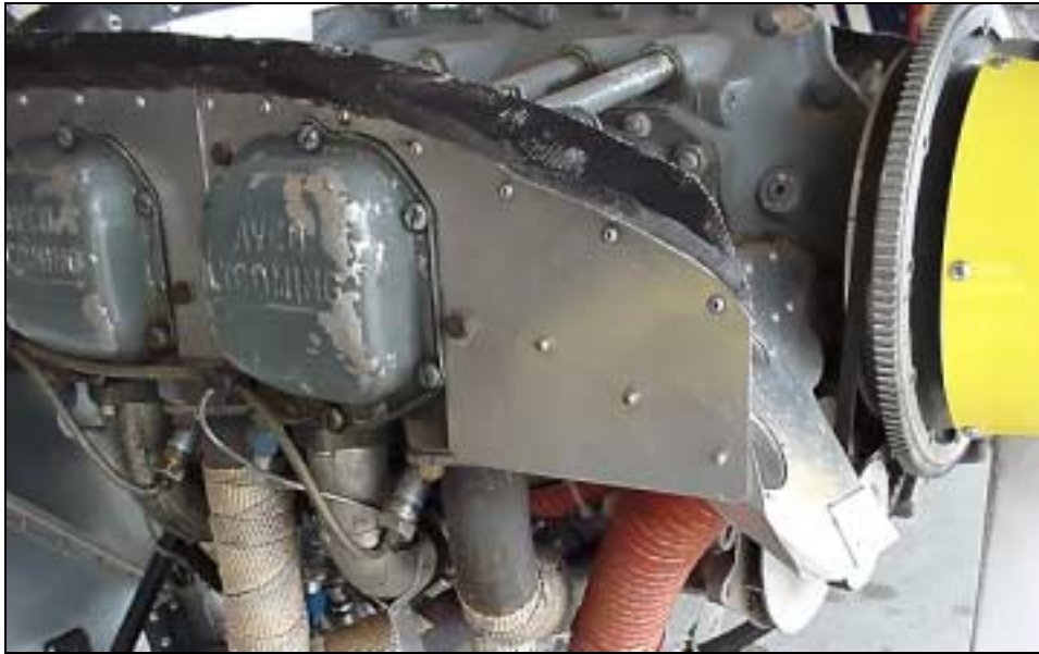
The right side baffle (installed).
