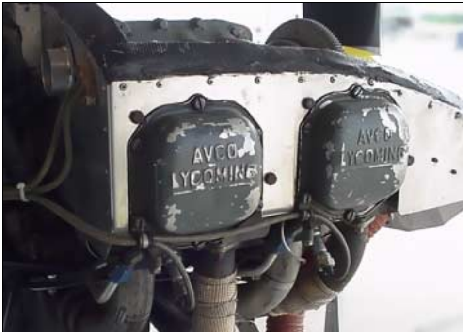
The right side baffle (installed)
