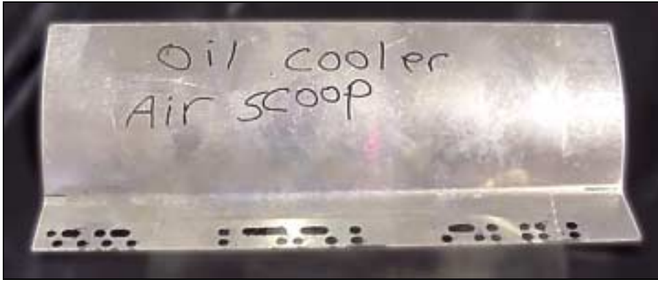
Oil cooler air scoop.
