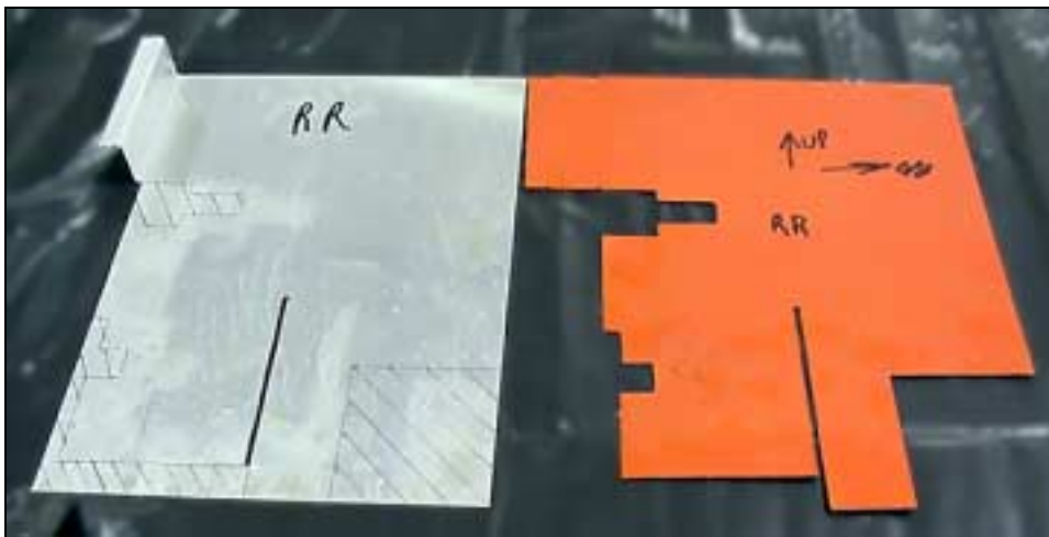
Right: the trimmed rear right (RR) baffle.
