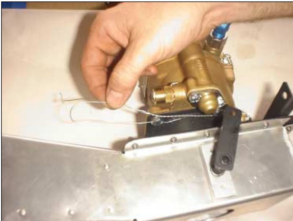
Wire is shown braided between the bolts.
