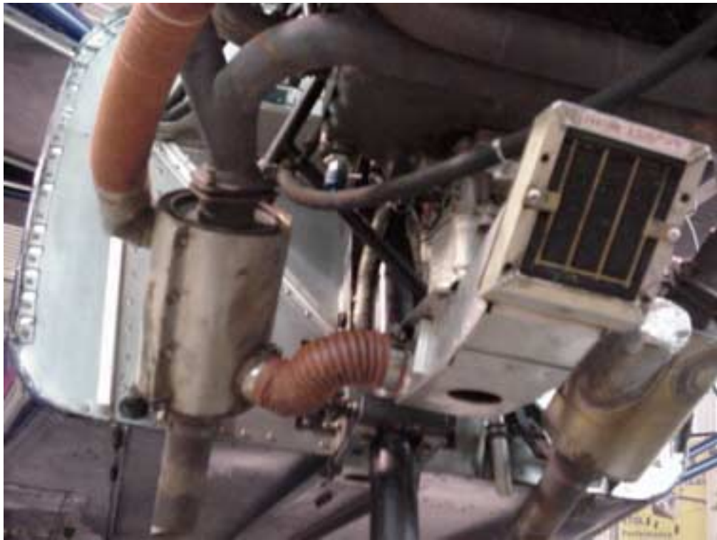
Carb. Heat Box, hole at the bottom is the hot air exit when carb heat is not used.
