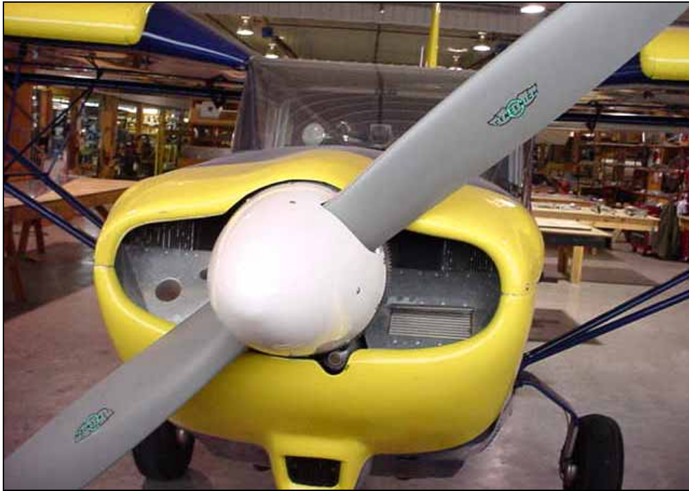
Spinner for the Lycoming 0-360 with a metal Sensenich propeller.
