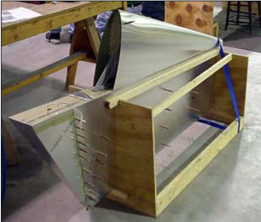
The rudder assembly in the wood jig with the strap.
