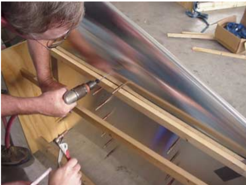
The rudder assembly in the wood jig with the strap.
