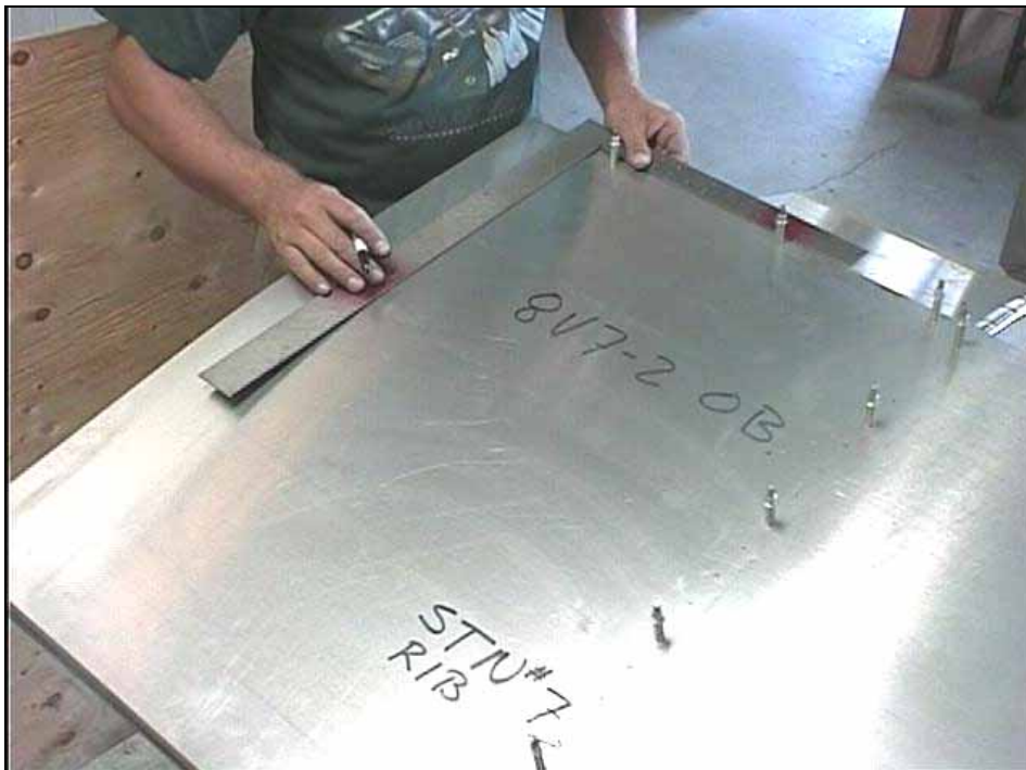
Photo shows marking the O/B skin for trimming.
