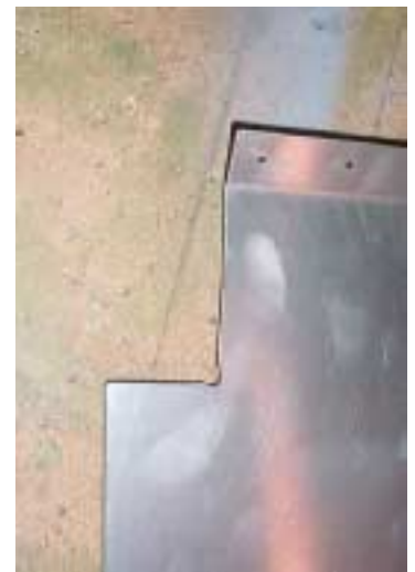
Detail of rear outboard cutout: 75x32mm
