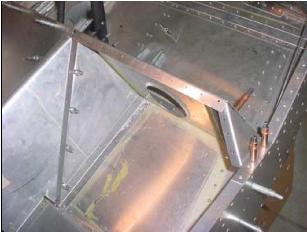
The aft flange rivets to the Seat
