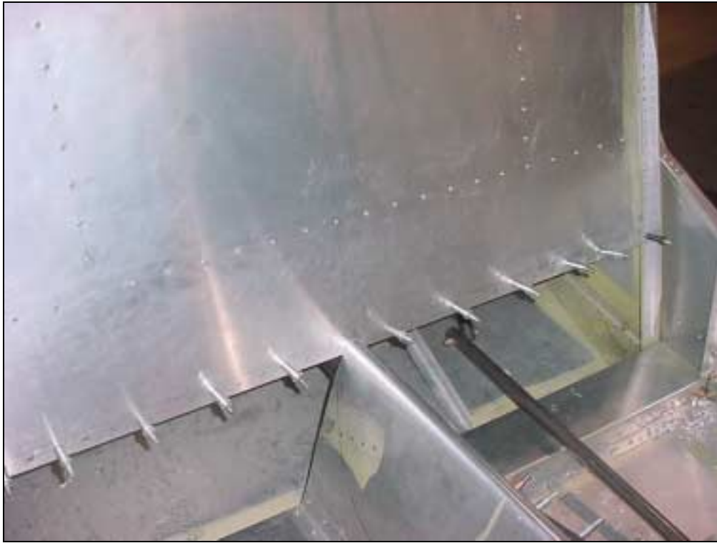
'L' Angle: length = 1025mm Clamp the 'L' Angle on the backside of the Seat back.
