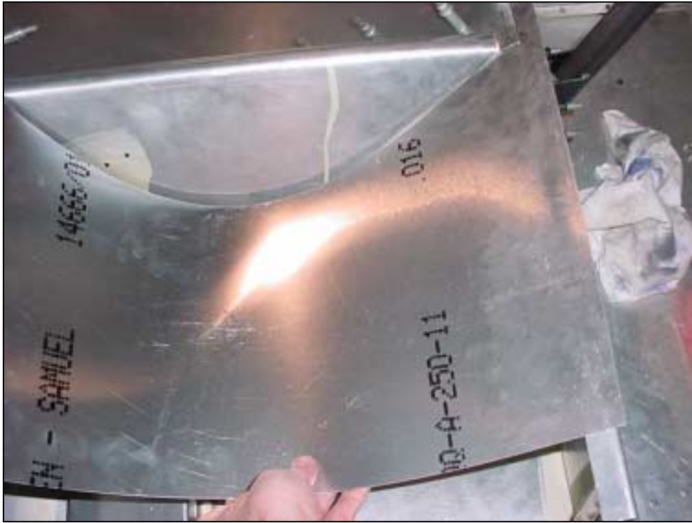
Trial fit template to determine the inboard cutout on the Seat 7F16-1
