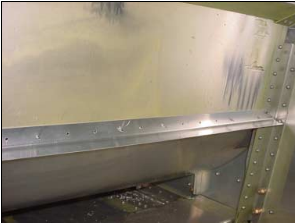
Viewed from inside the fuselage looking forwards. 'L' Angle along the bottom of the Seat Back. ORIENTATION: the bend is towards the bottom.
