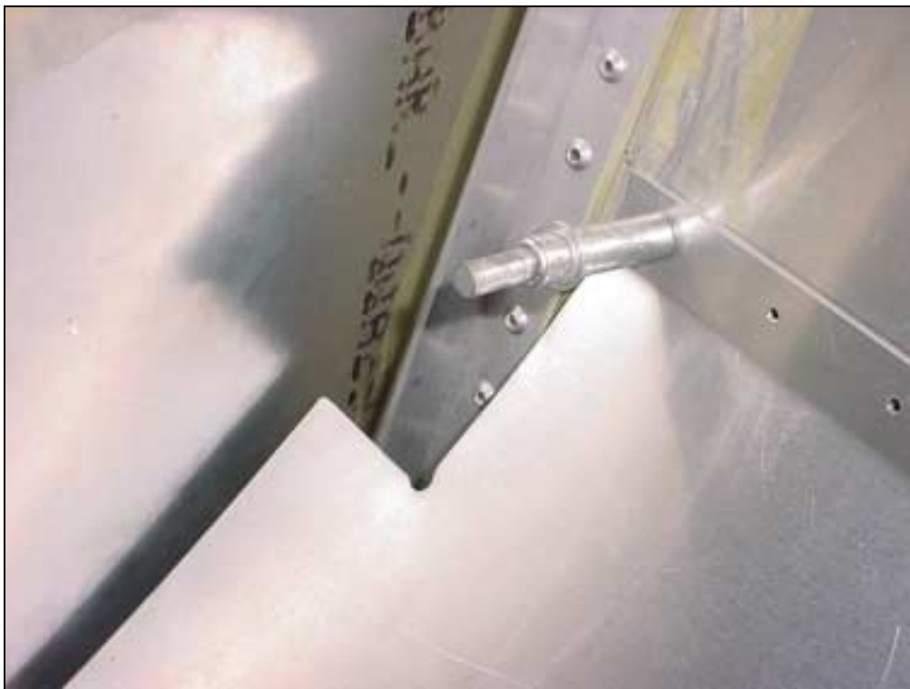
Detail of rear outboard cutout: 75x32mm
