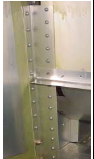
The ends of the 'L' Angle overlap on top of the Upright 7F11-5
