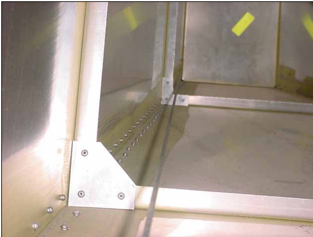
Photo of right side, bottom left and right Gusset (first Gusset in front of the Front HT Frame 7F1-4) cutout to make room for rudder cables. The Gusset is trimmed flush with the 'L' Angles.
