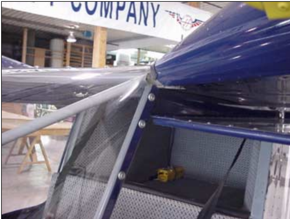
The top screw also picks up on Door Sill 7F19-12D
