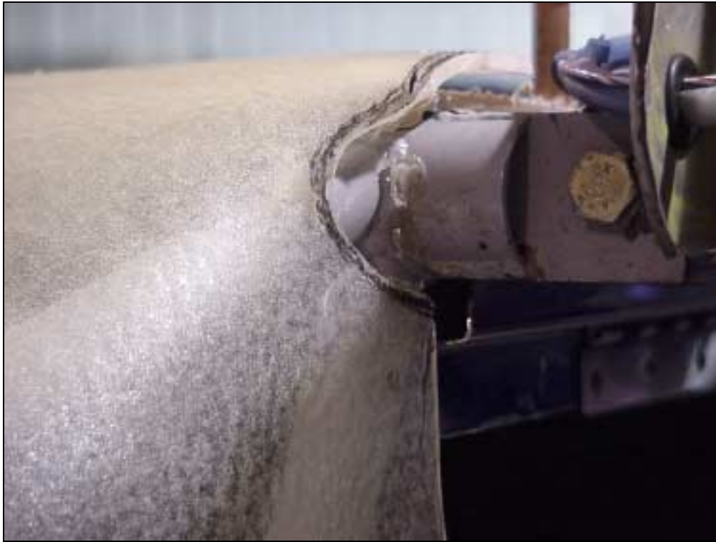
Detail of the Windshield around the main Wing Spar attachment with the Cabin Frame
