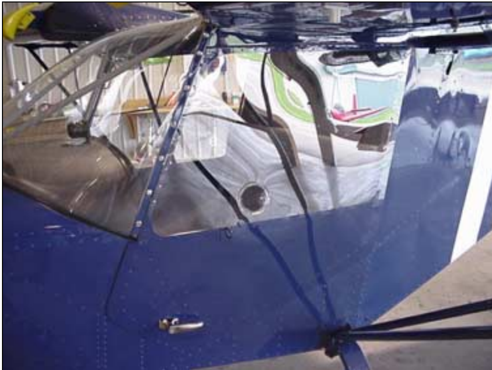
The Door Side 7F19-7D is even with the bottom aft corner of the Windshield.
