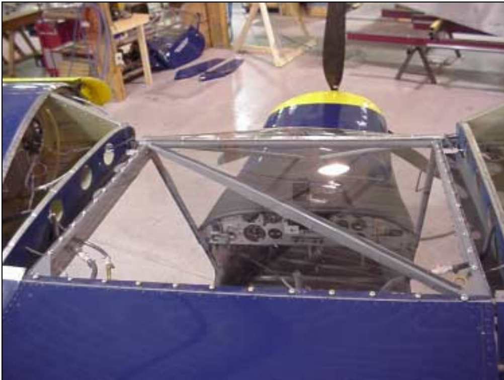
The Windshield can also be installed with the Root Skin 7V9-1 removed
