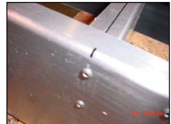
Rib station reference line on spar.
