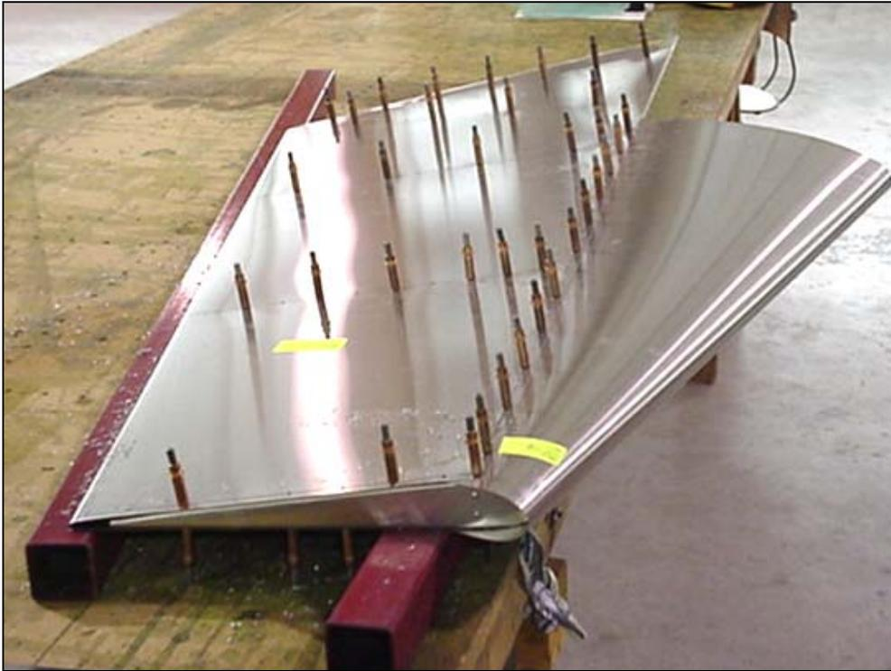
Before drilling make sure the Rudder is correctly positioned on the boards or beams with the spacer under the bottom trailing edge. Start drilling from Nose Rib working towards each end and Cleco every other hole. Drill both sides.
