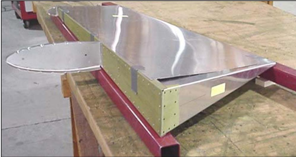
Position the skeleton inside the skin; line up the reference lines, adjust the front of the skin flush with the spar.
