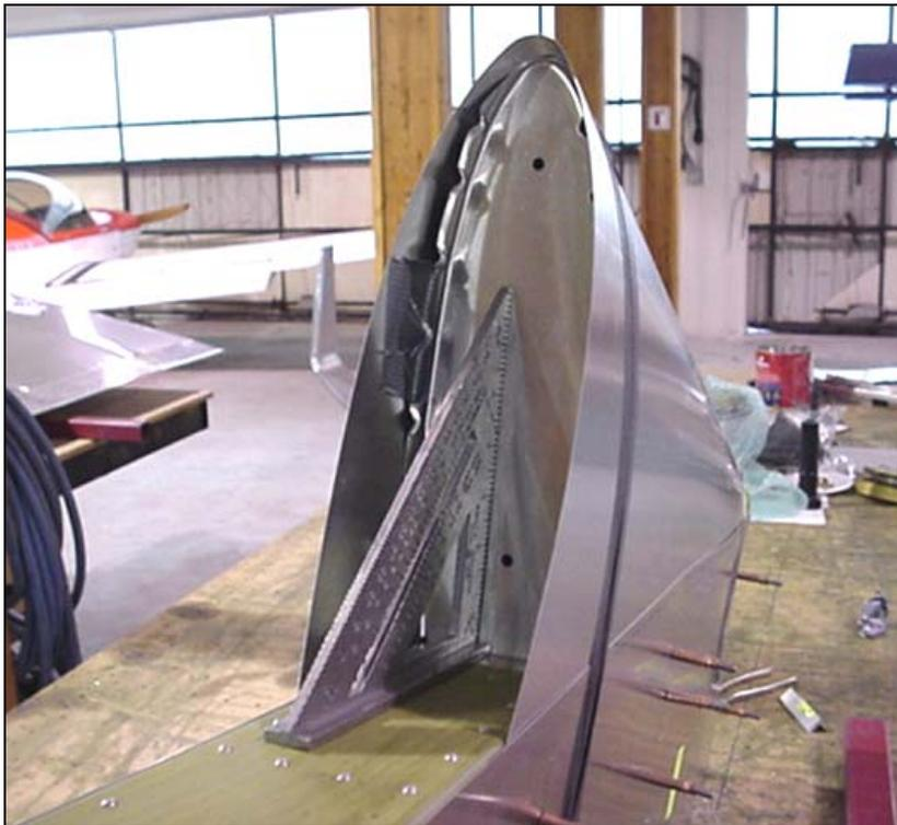
The Nose Rib is at 90 degrees to the Spar. Verify that the center of the Nose Skin radius lines up with the center of the Nose Rib radius.
