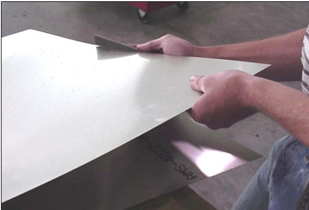
File the edge to remove any slivers or jagged edges and burrs. The final test is to run your finger over the edge, do not attempt this before filing.
