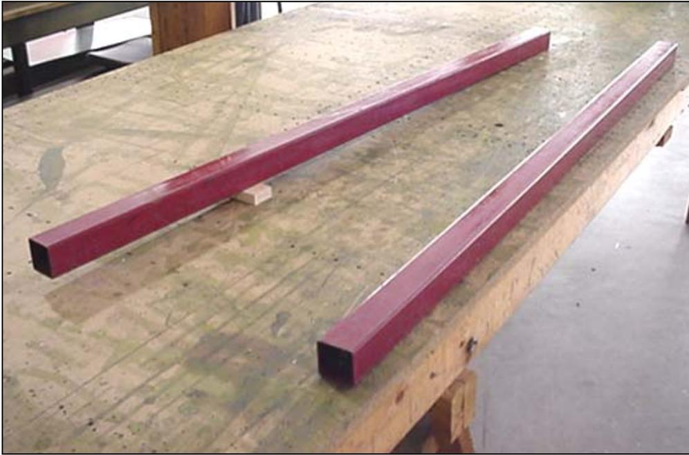
Square 2x2 steel beams (4ft long). Straight wood boards, such as a 2x4, can also be used instead of the steel beams.
