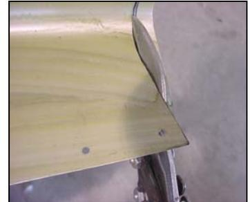
Cut the top of the Nose Skin flush with the Tip Rib. First do a couple of rough cuts to practice holding the snips “up side down” to work around the leading edge.
