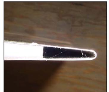
The end of the tip rib may not be supported on the beam, be careful not to push down too hard.
