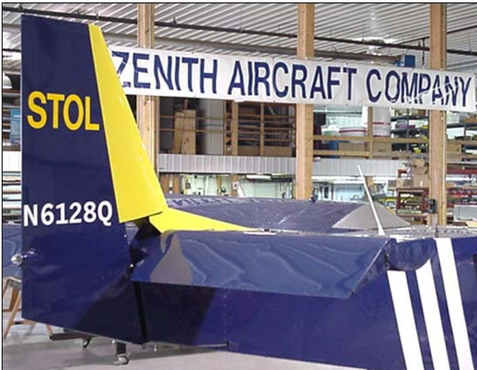
The finished STOL rudder assembly installed to the aircraft
