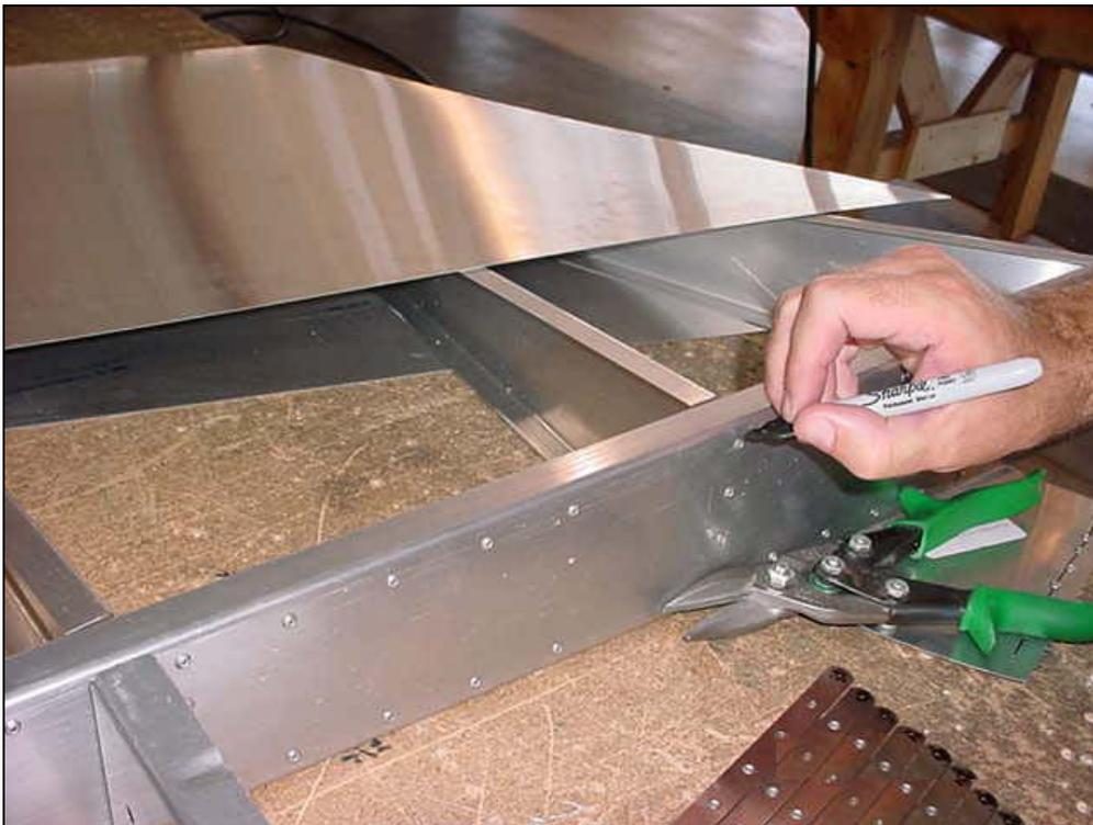
**REFERENCE LINES:** Extend the rivet line through the rib flange to the edge of the spar, for ribs #2, 3 and 4.
