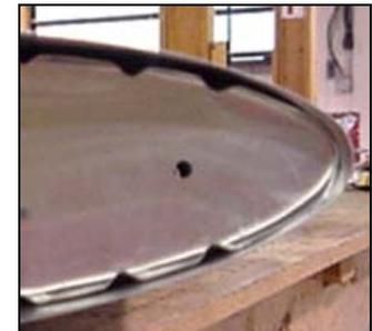
**CHECK:** Make sure there is no gap between the leading edge of the ribs and the nose skin.
