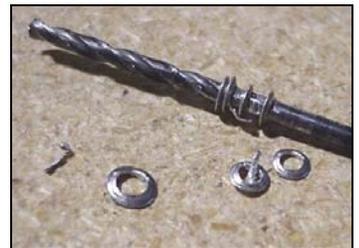
Drilled-out rivet heads. Pull a new rivet in the hole.
