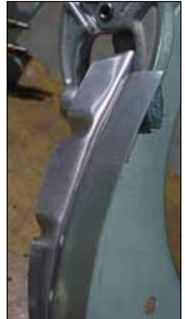
Clamp the bent L angle to the rib.
