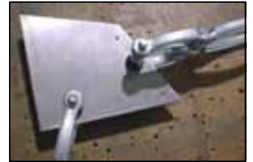
Use the first slat support to drill the other 4 (4 total per wing).
