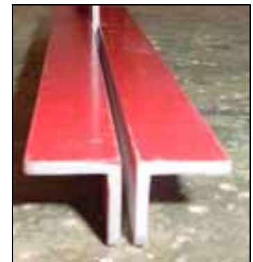
Instead of making a separate template for the left and right side, two pieces of extrusion are riveted with the plate in the middle.
