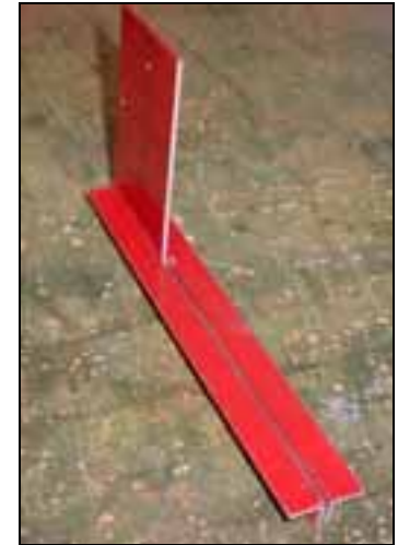
Clamp the plate at 90 degrees to the extrusion.
