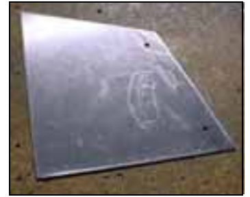
7V4-5 Slat Supports. Layout and drill the two holes with #40 holes.
