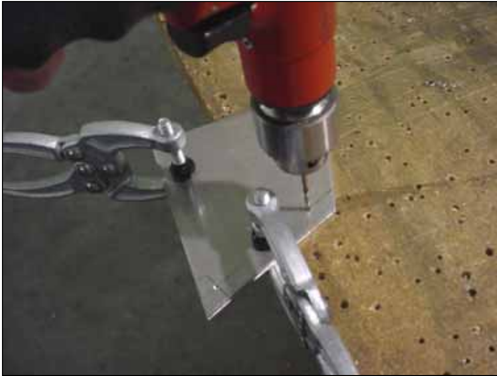
Clamp 2 slat supports together, back drill through the pre-drilled holes.
