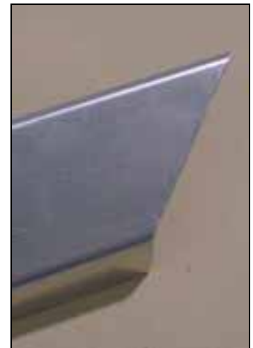
Detail of bottom flange, end is cut square to the aft edge.
