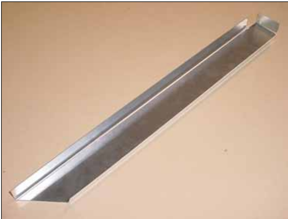
Detail of bottom flange, end is cut square to the aft edge.
