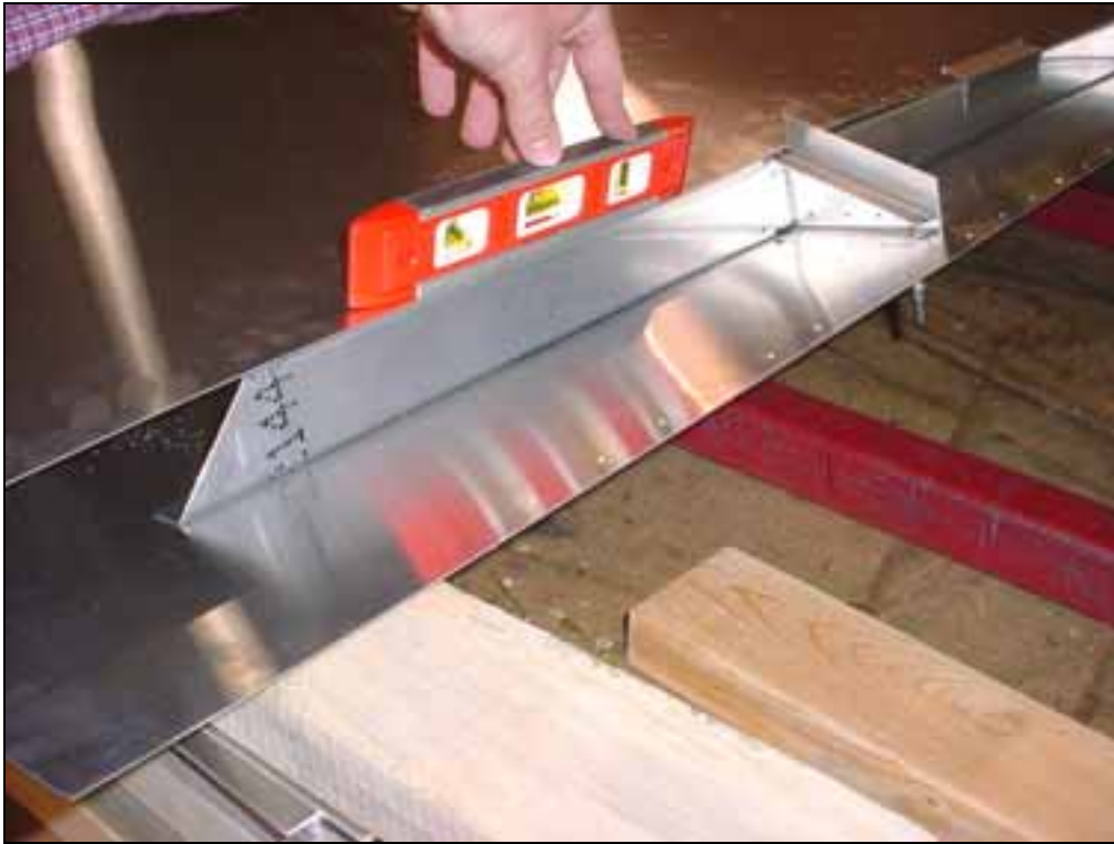
Level the inboard end of the heavy rear channel 7V6-1
