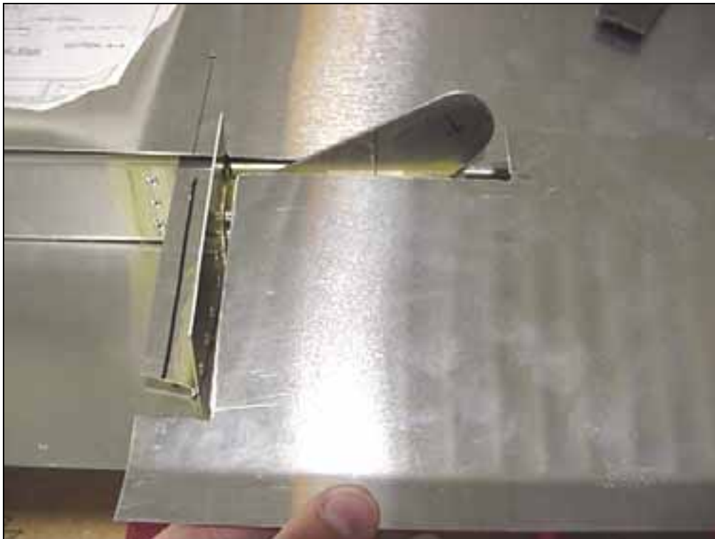
Cutout to make room for the rear strut attachment and bracket.
