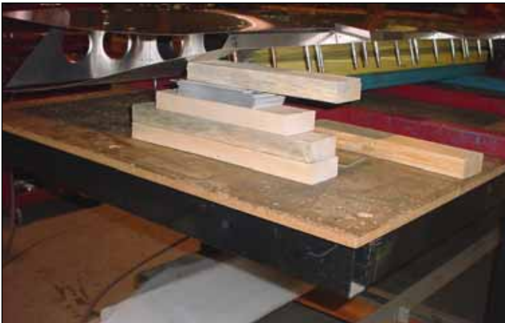
If necessary, build up space between workbench and side of wing to level the channel.
