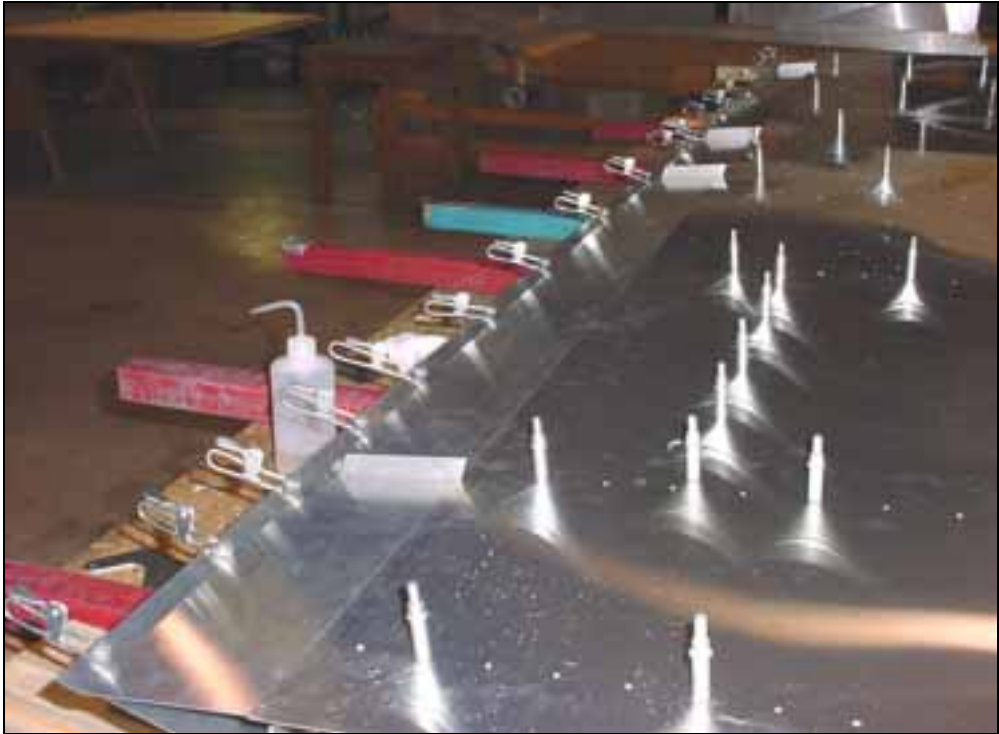
Clamp the trailing edges flush.
