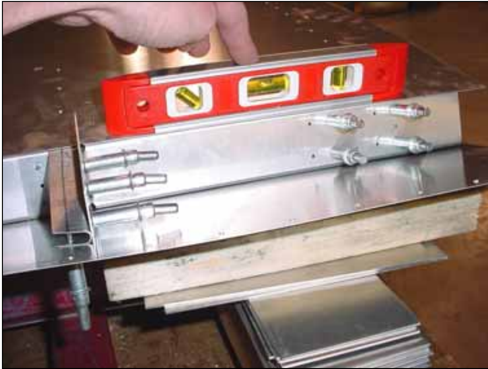
Level the ends of the rear channel. Detail of the outboard end.
