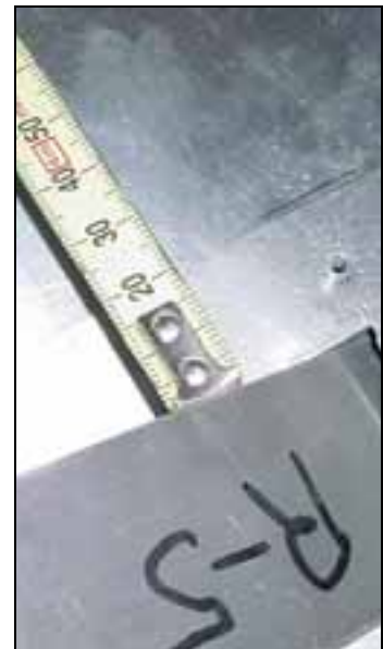
Zero reference: aft edge of the strut fitting. Ref. middle diagram on drawing 7-V-8
