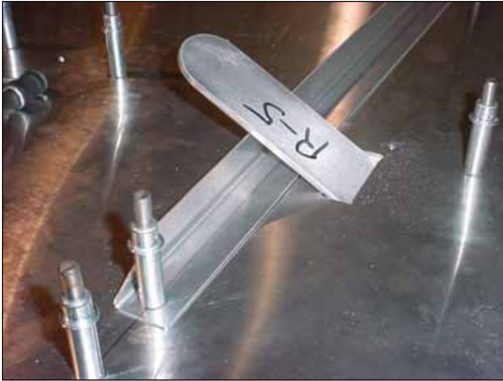
Drill and Cleco the front end hole.
