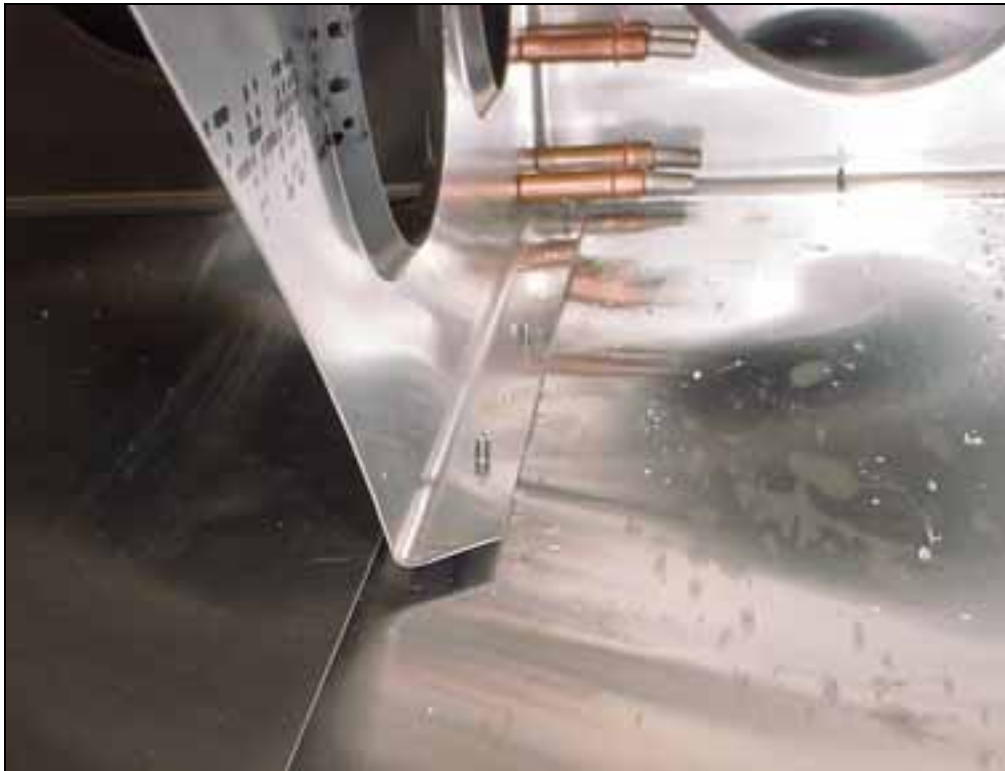
Check the rivet line is in the middle of the flange.
