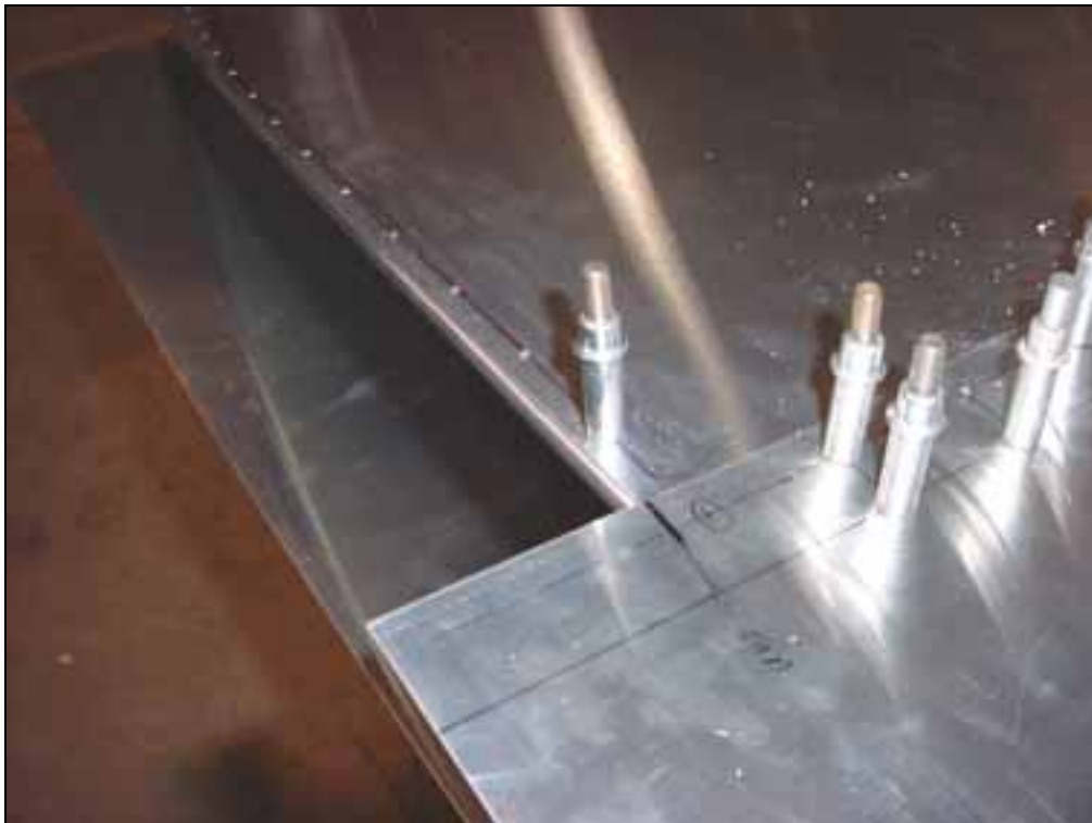
Line up the bend tangent line (beginning of the radius) on the edge of the skin.
