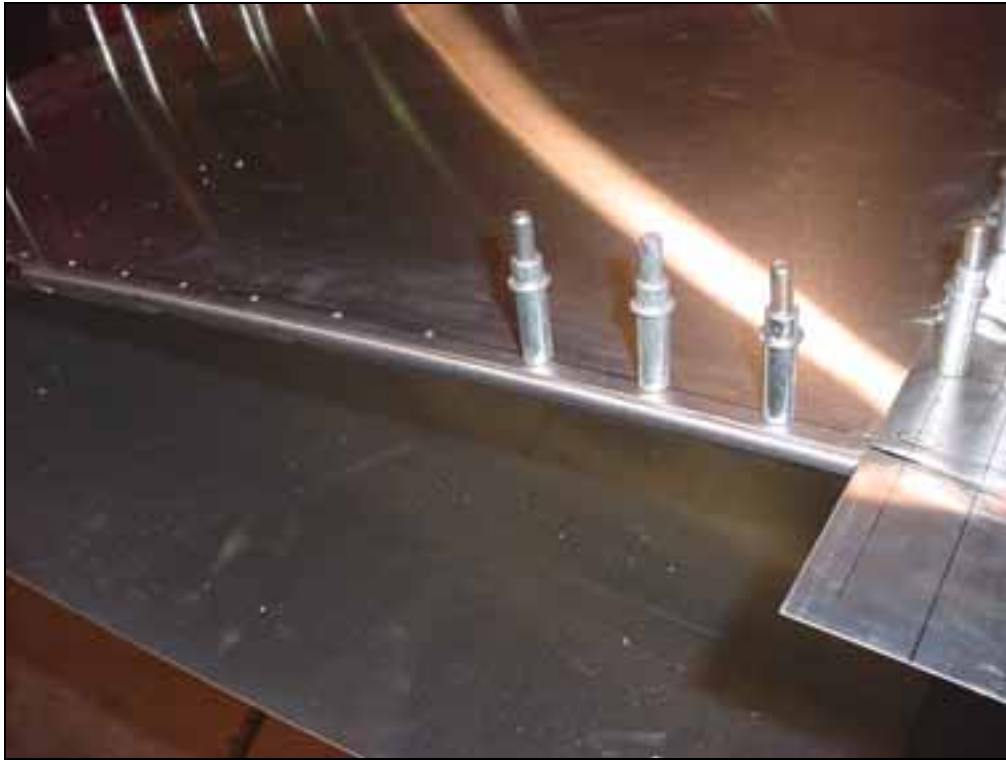
Detail: location of crimp between the rivets.
