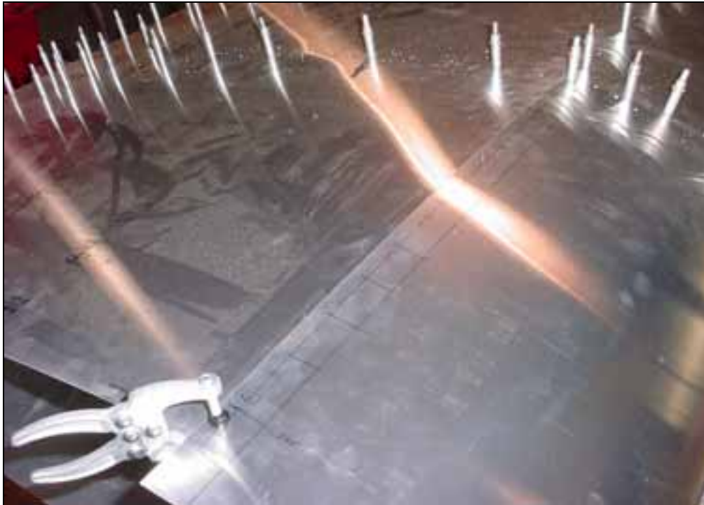
Clamped. End hole is 10mm from the end of the spar tip.
