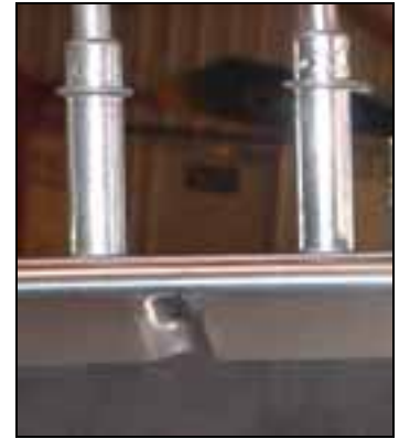
Detail: location of crimp between the rivets.
