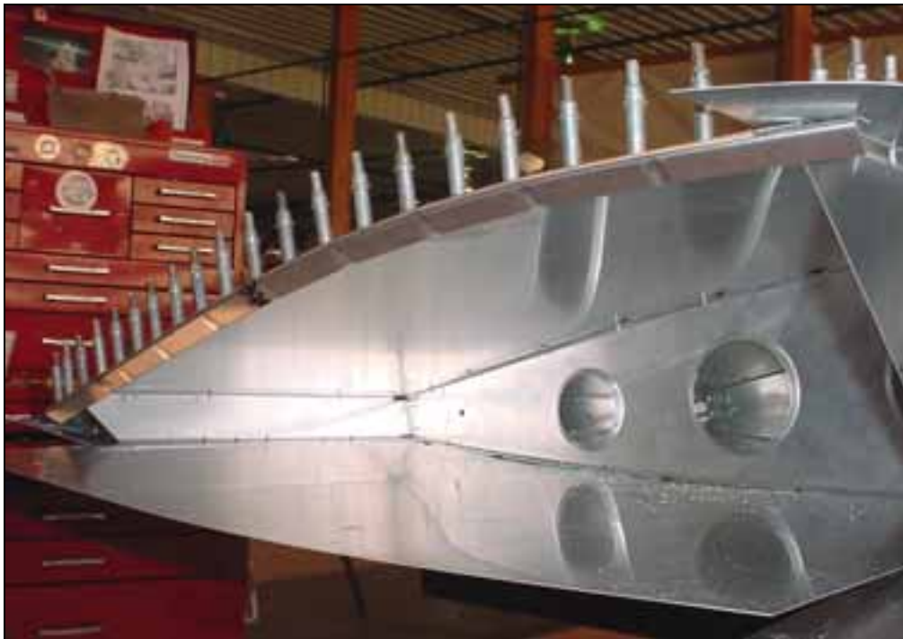
Top tip angle 7V8-2 Clecoed to the top skin 7V7-2
