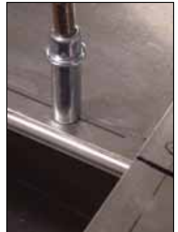
Line up the bend tangent line (beginning of the radius) on the edge of the skin.
