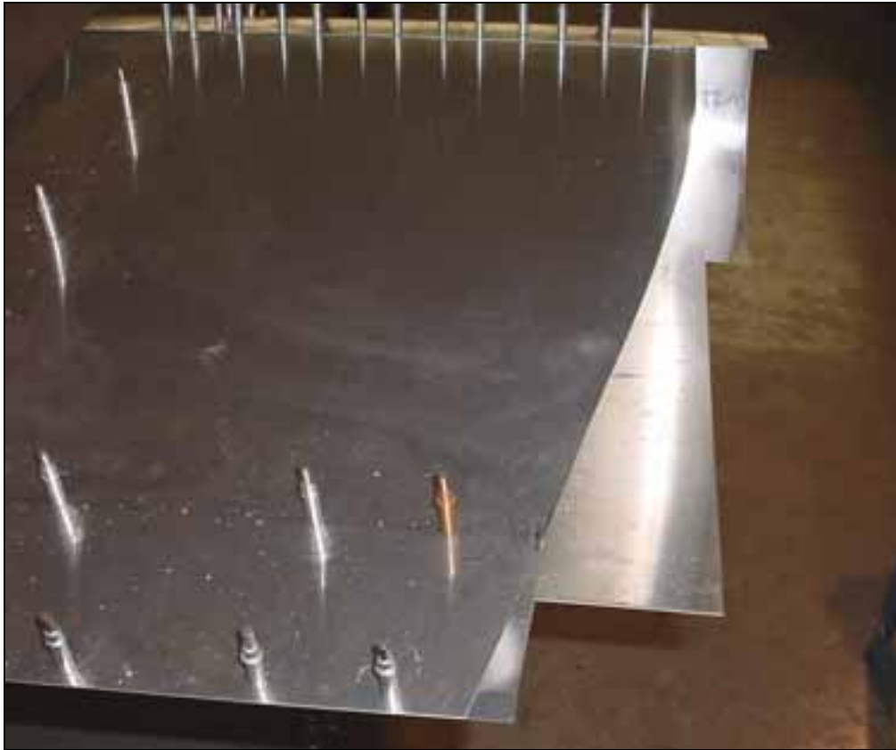
7V7-2 Rear Top Skin (Right wing, view from rear). Trim on line, file to a smooth edge.
