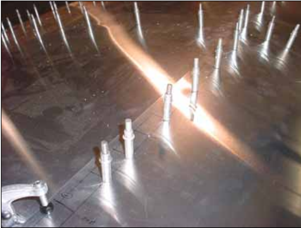
Drill and Cleco the front rivet line through the spar tip 7V3-3.
