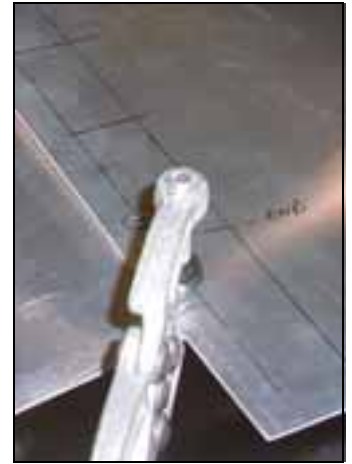
Clamped. End hole is 10mm from the end of the spar tip.
