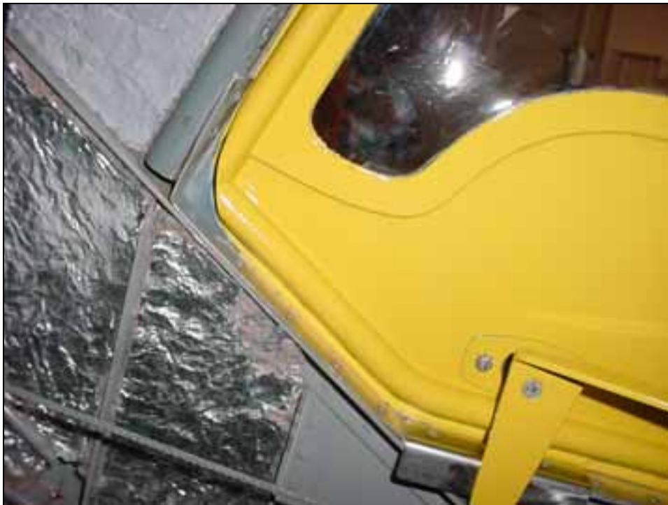
Front bottom reinforcement in fiberglass door has to be trimmed to fit the curvature of the door opening on the fuselage.
