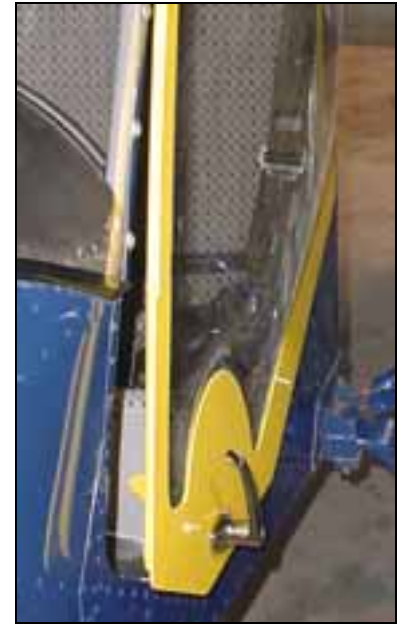
Door springs open, door in the unlatch position.
