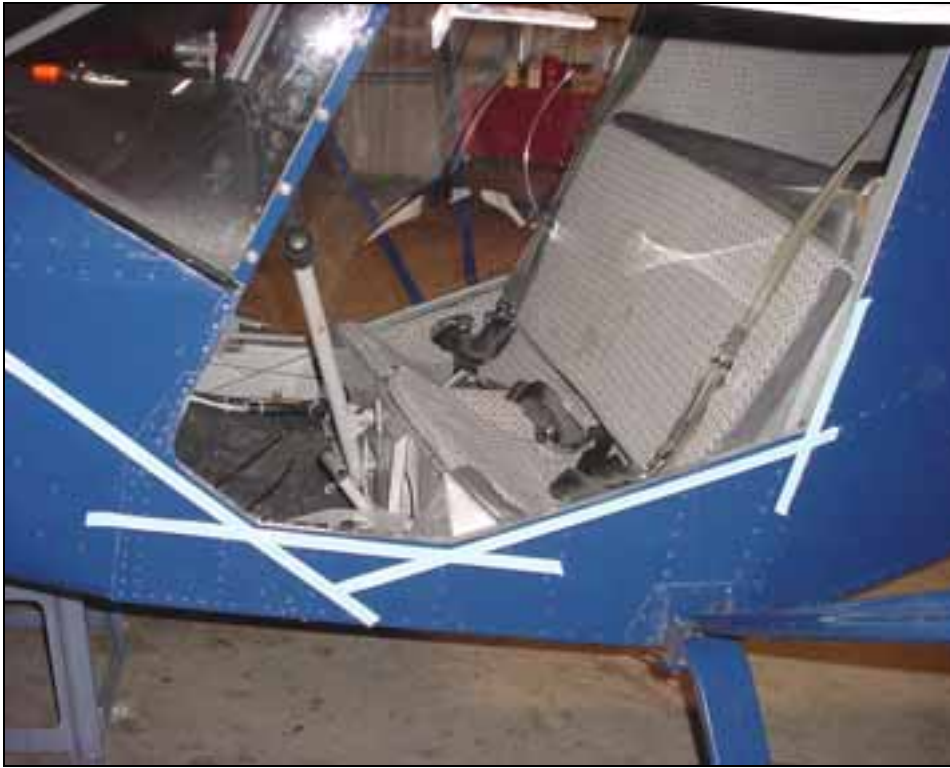
Stick long strips of tape along the top edge of the solid rivets in the cabin frame.
