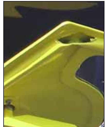
Grind away the reinforcement frame to fit the door inside the opening in the fuselage.
