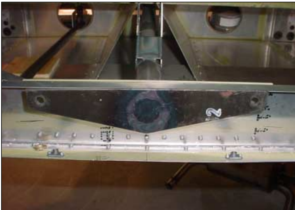
The top of the Horn 7C2-3 is installed square to the side of the Torque Tube.
