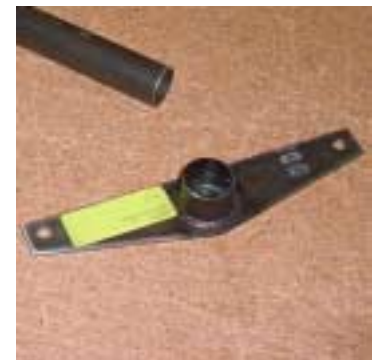
Drill the two 5/16" hole for the Bolt AN5.
