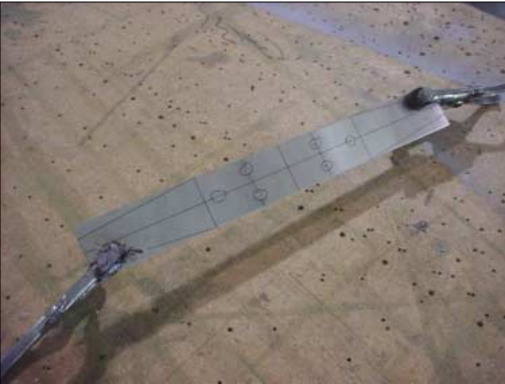
LAYOUT: Mark the centerlines and shape of the part. Layout the holes and the 6 rivets.
