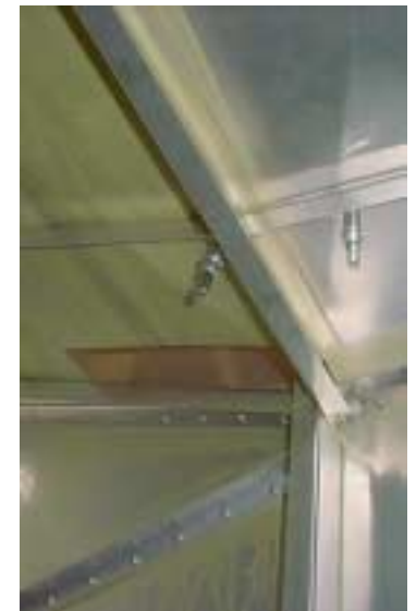
Photo of left side. 'L' angles on the front and aft side of the Zee Channel 7F8-10B
