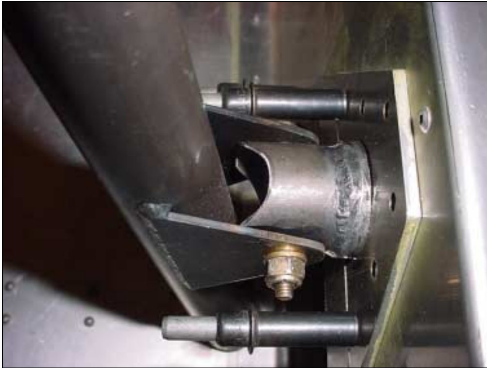
Front Bearing Top 7F11-2 on the backside of the stop ring welded on the Torque tube 7C2-2.
