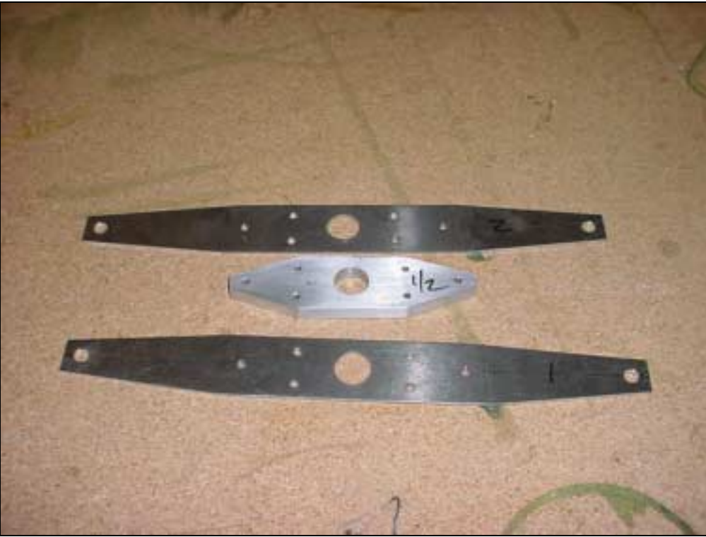
Part after they have been cut, drilled and deburred
