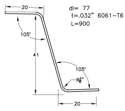
ADDITIONAL REINFORCEMENT Z ANGLE WHEN 7F5-3 OR 7F5-3SP IS t=.040" (NOT REQUIRED IF 7F5-3SP IS t=.063")
