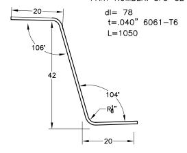
ADDITIONAL REINFORCEMENT Z ANGLE WHEN 8F5-3 IS t=.040" (NOT REQUIRED IF 8F5-3 IS t=.063")
