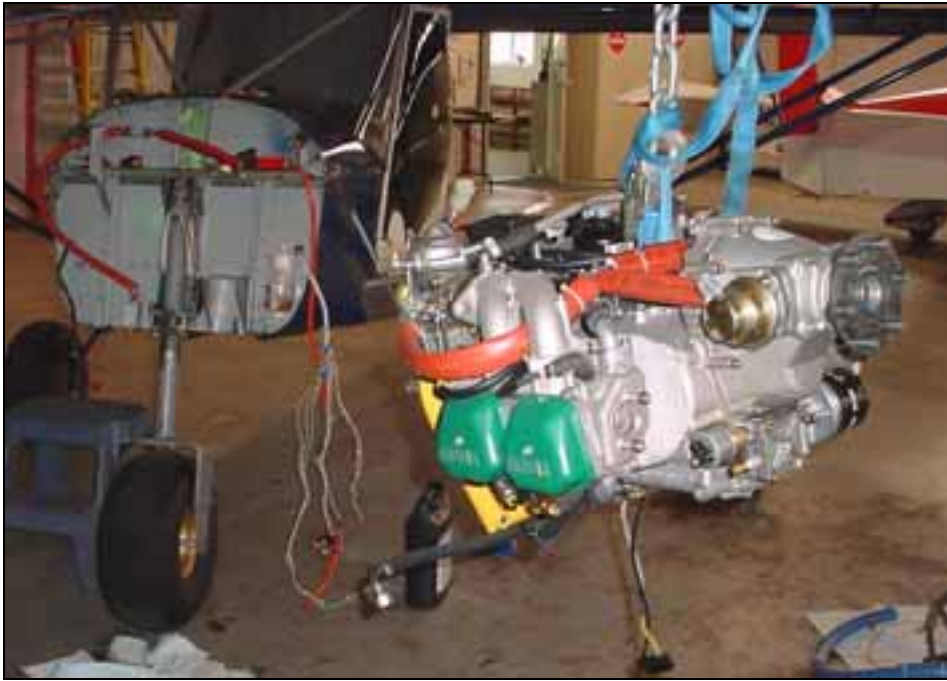
Engine hanging from engine hoist.
