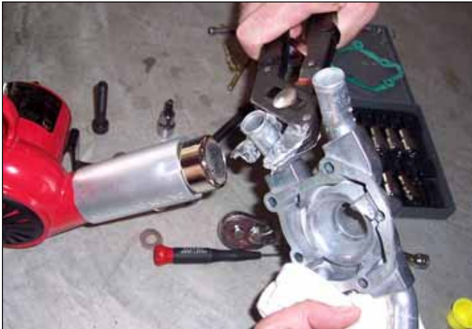
Allow the water pump housing to cool. Then test fit the water pump housing to check the clearance between the fittings and the Ring Mount.
