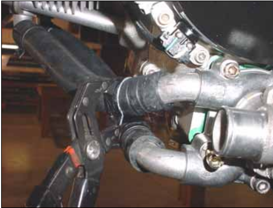
Remove the 4 hose from the water pump.
