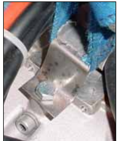
Strap across the steel bracket to the chain.
