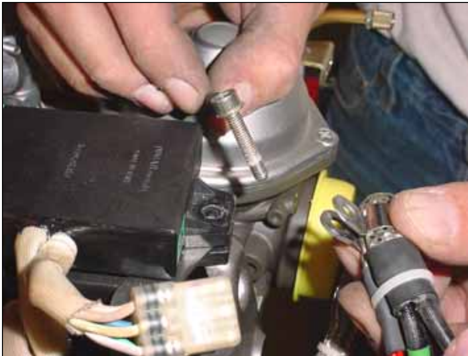
Remove the top Allen screw on top of the ignition coils.
