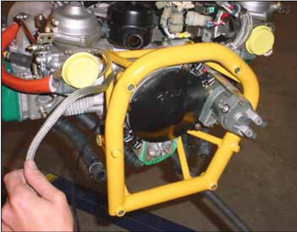
Feed the cable through the top left tubes.
