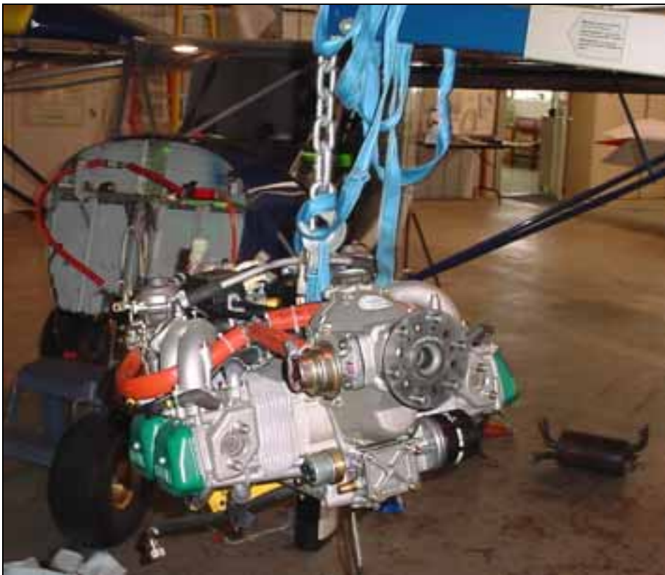
Getting engine read to install the Rotax ring mount.
