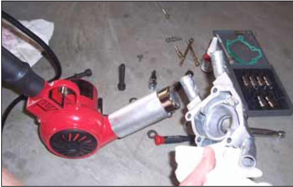
Fittings on the left side of the water pump housing point at the supports for the Ring Mount.
