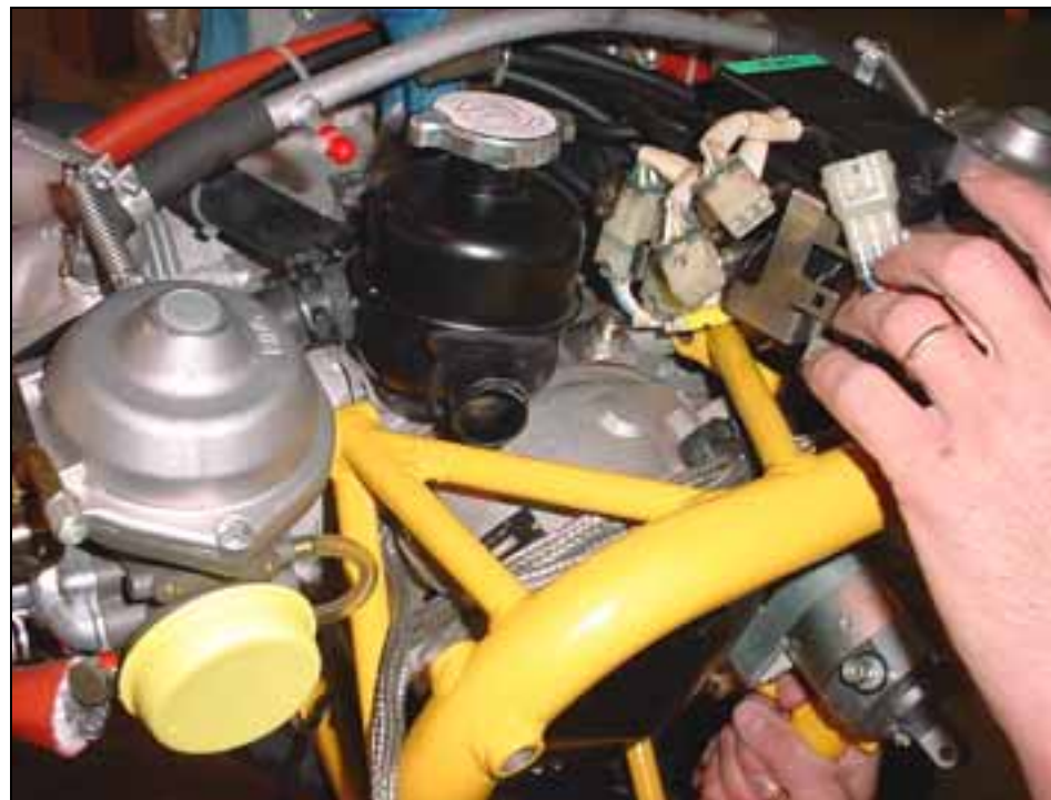
Line up the ring mount with the tapped holes on the side of the engine.
