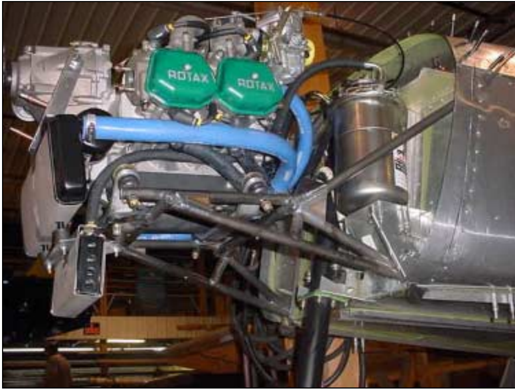
Left side of engine Oil line from top of the tank to top left side of oil cooler
