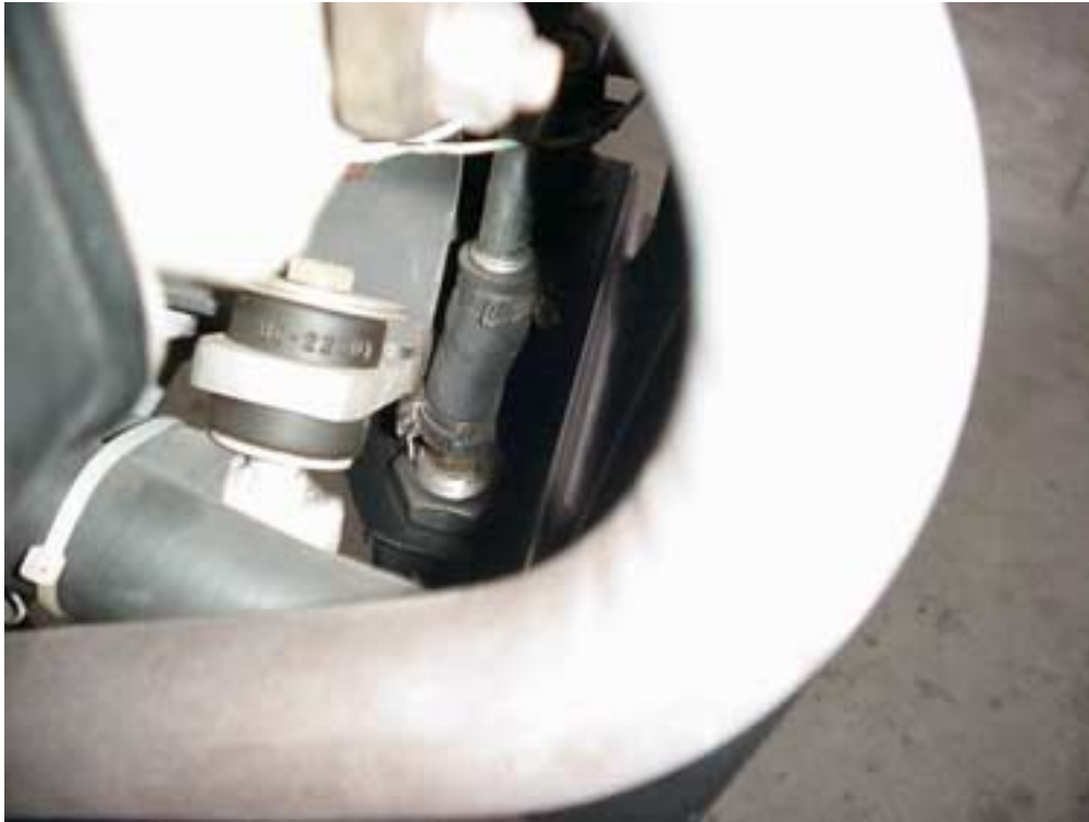
Detail of right side fitting to oil cooler.
