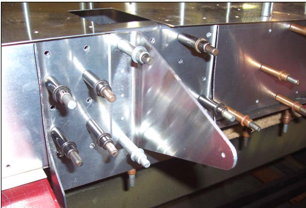
Cleco the Center Hinge Bracket to the Rear Bracket and Rear Spar. (The Horizontal Stabilizer is right side up in this photo.)
