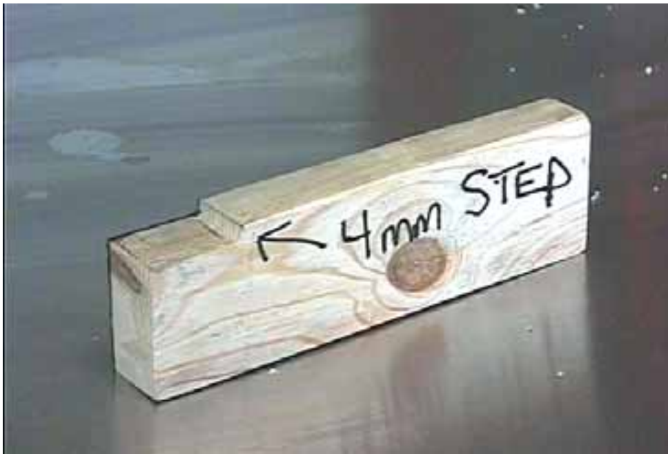
Joggling stiffeners. 4mm step approximately 15mm long.
