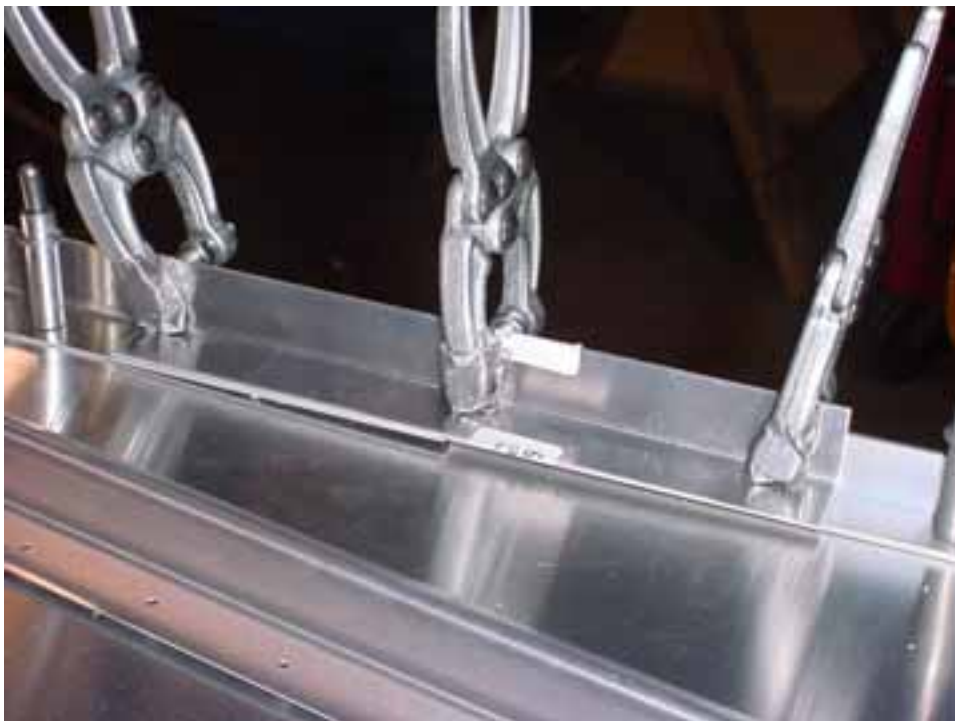
Position the Doubler 6B2-2 on top of the shim. Check there are no gaps between the parts.
