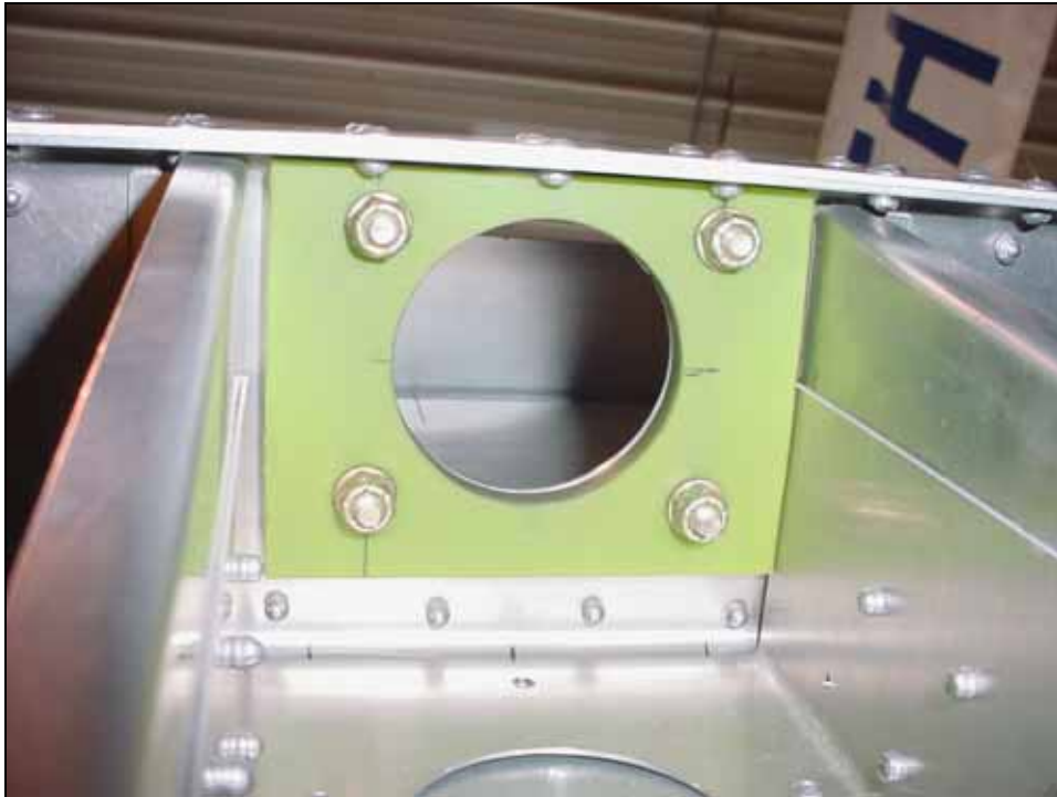
Nylon self locking nuts and washer. Looking up at the upper bearing 6B8-6
