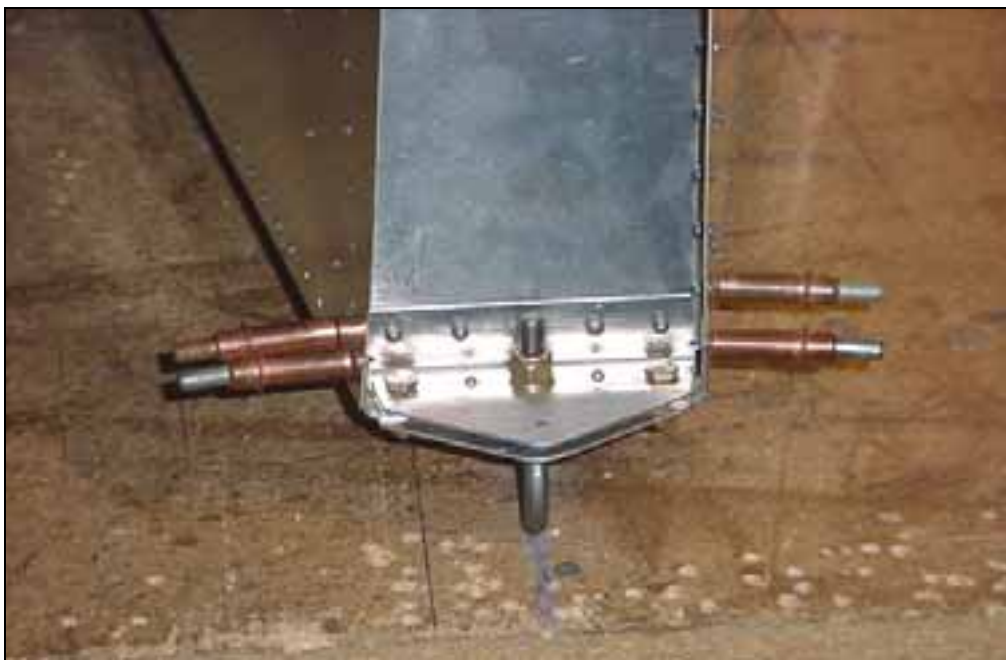
Detail of chalk line and aircraft center at the rear of the fuselage (tie down ring 6B4-1).
