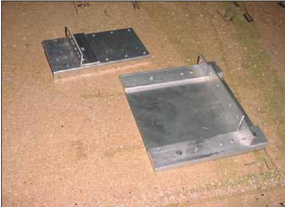
Spar insert and rear channel assembly ready to be clamped to spar web.
