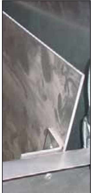
75mm from top of web template to top flange of rear channel.
