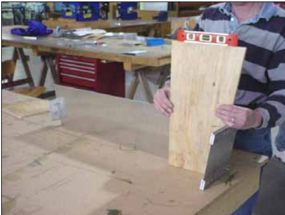
Clamp the spar insert to the web template. Check angle. Drill and Cleco.
