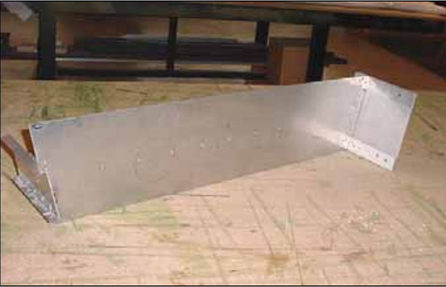
Wing Jig fit for left side, photo to show inboard side.
