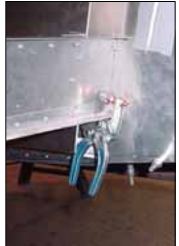
Detail of back side of wing jig: rear channel overlaps on the back side of the attach plate 6B5-4
