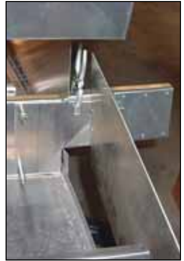
Clamp the attach plate 6B5-4 to the rear channel.
