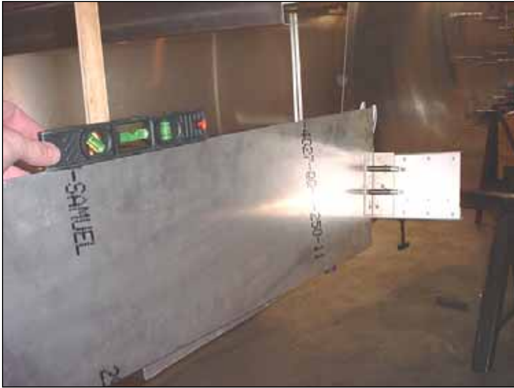
Level the top of the web template.
