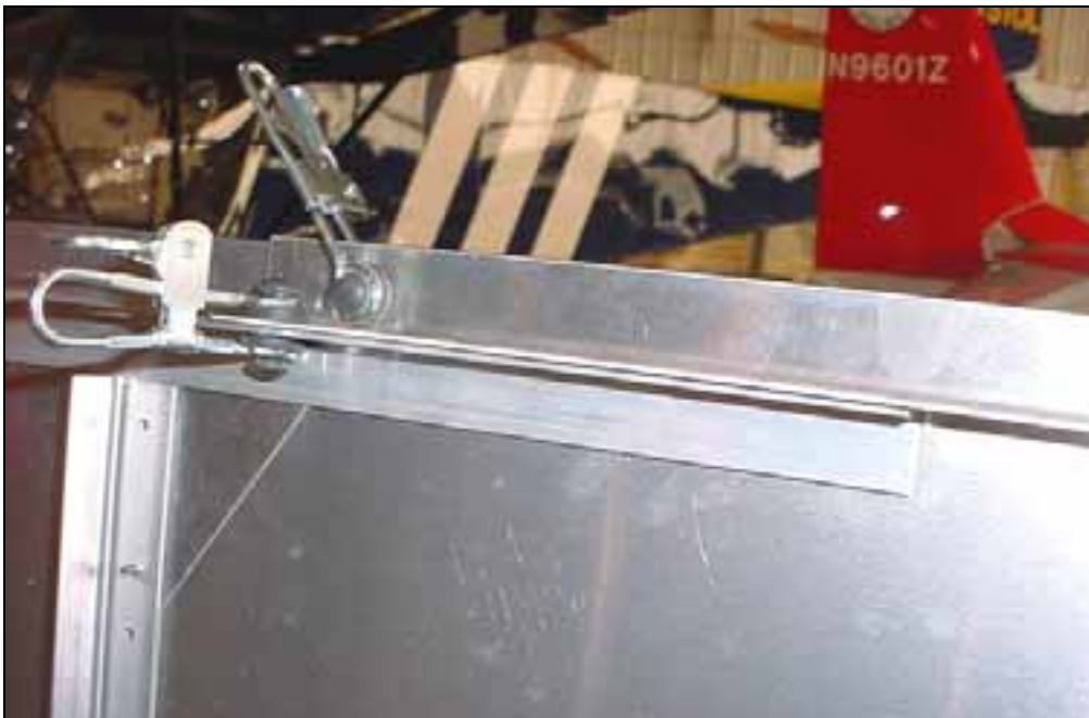
Longeron splice detail: Longeron 6B11-1 underneath rear top longerons 6B2-1 Photo of right side looking forward.
