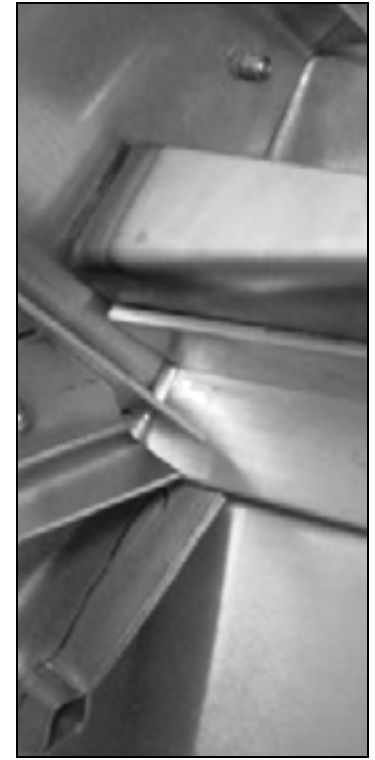
Inside view: check that the front of the longer overlaps the firewall flange.
