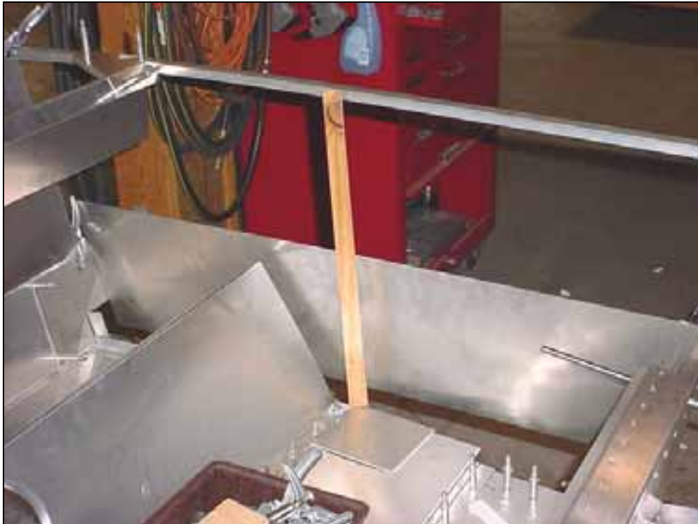
Inside view of the left wing jig.
