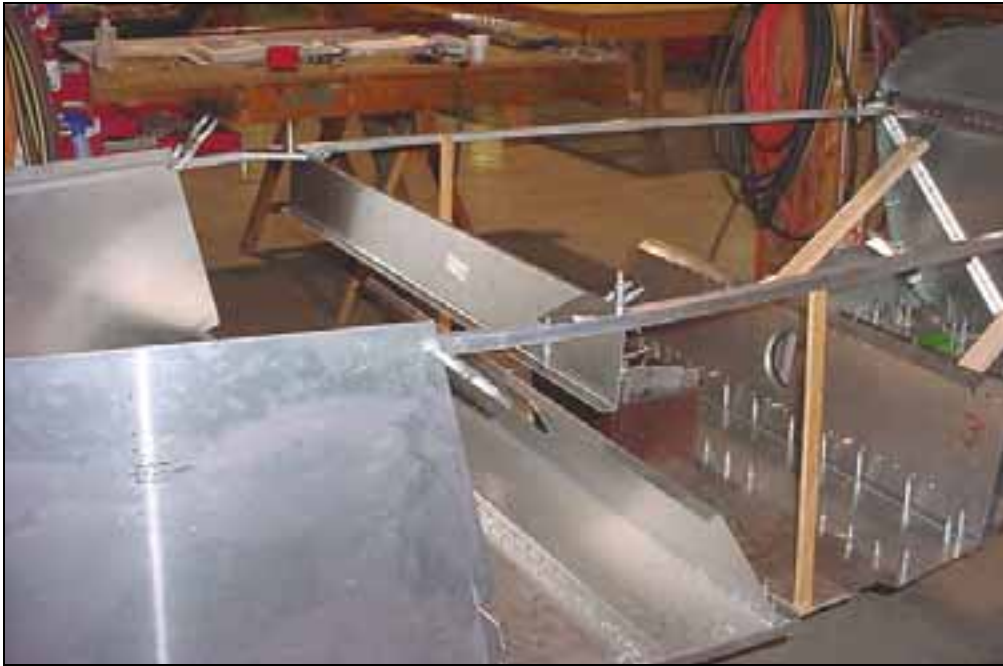
Rear fuselage with seat support 6B16-6 installed. Photo looking forwards.
