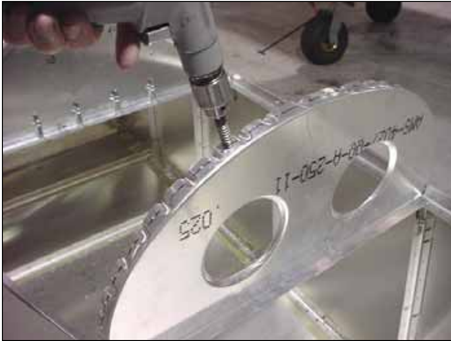
25 PILOT HOLES IN 6B12-1
