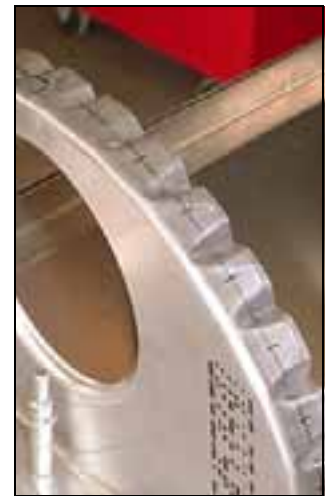
Layout the rivet spacing between the crimps.
