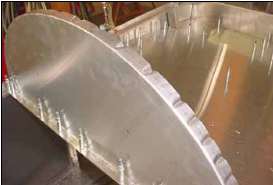
31 PILOT HOLES IN 6B12-2
