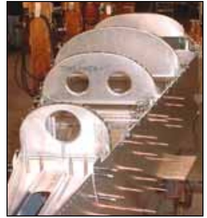
Bulkheads on fuselage.
