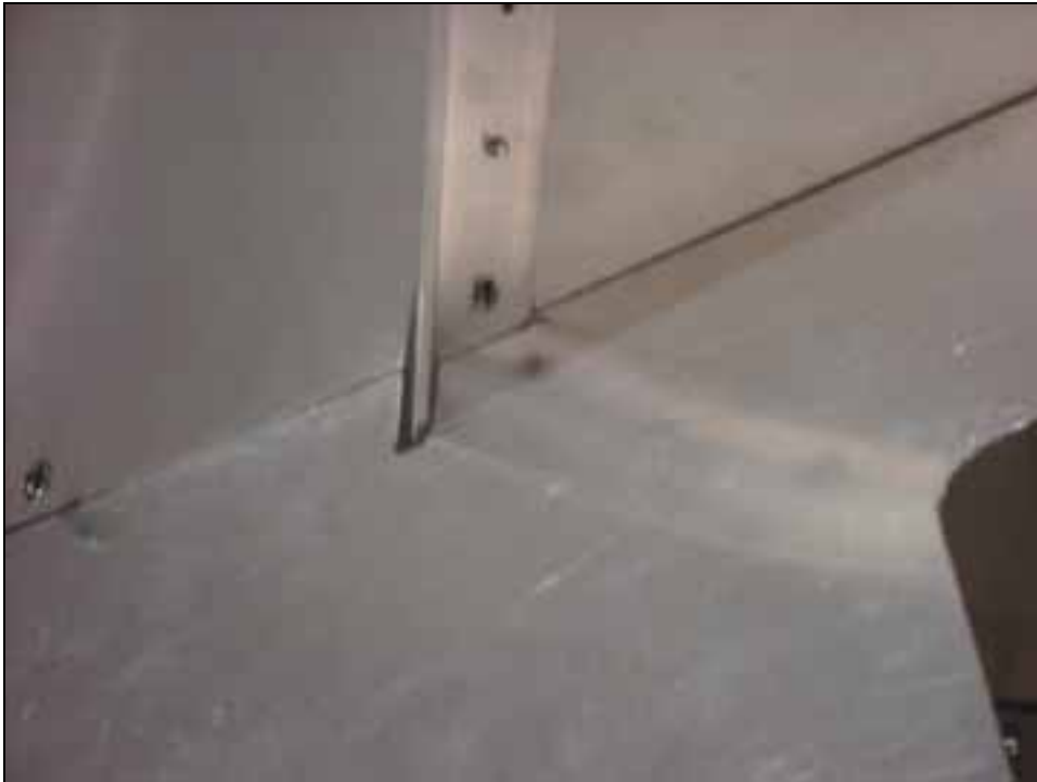
Cutout in the Seat Panel to make room for the Gear Upright 6B11-3
