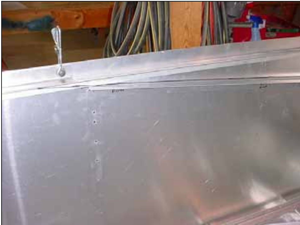
End of diagonal L angle even with aft edge of vertical L angle.
