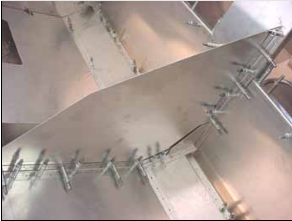
SEAT BELT ATTACHMENT DOUBLER PLATE 6B18-3
