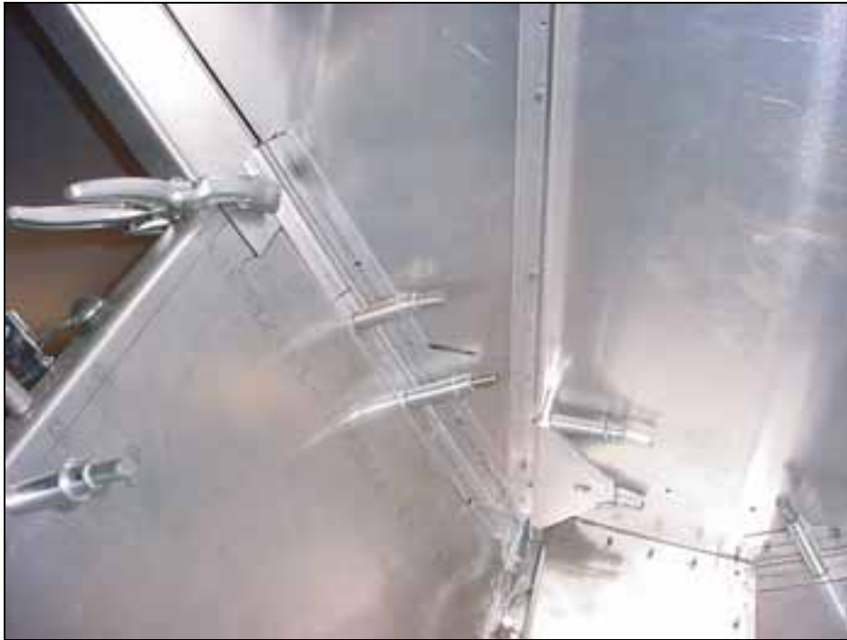
Left side: Note the no rivet zone for the flap mount gusset 6B19-9
