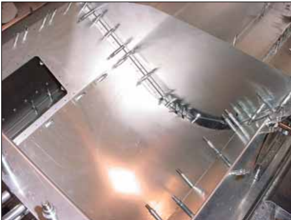
A5 PITCH 25 Front: 6B18-6 into 6B15-5 Rear: 6B18-6 into 6B5-1
