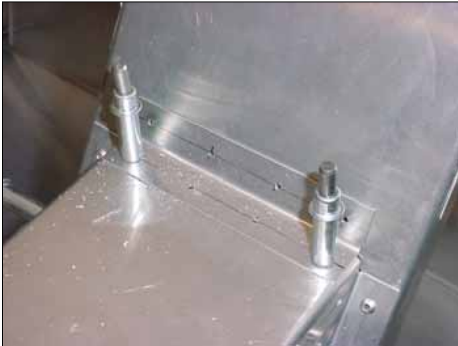
L angle in the corner of the arm rest cover 6B18-2 and the center seat back channel 6B16-2
