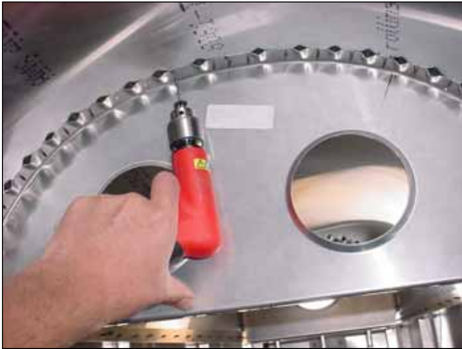
The middle bulkhead is back drilled by reaching in through the bottom fuselage access door 6-B-3
