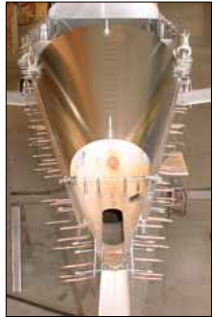
Tape both sides of the top skins to the sides of the fuselage.
