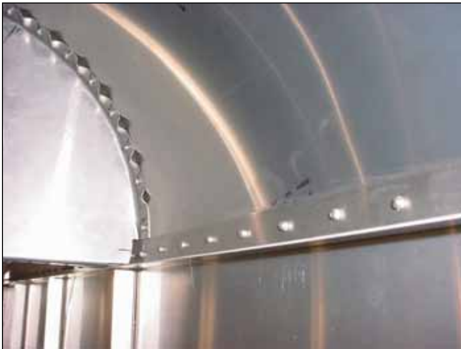
The middle bulkhead is back drilled by reaching in through the bottom fuselage access door 6-B-3
