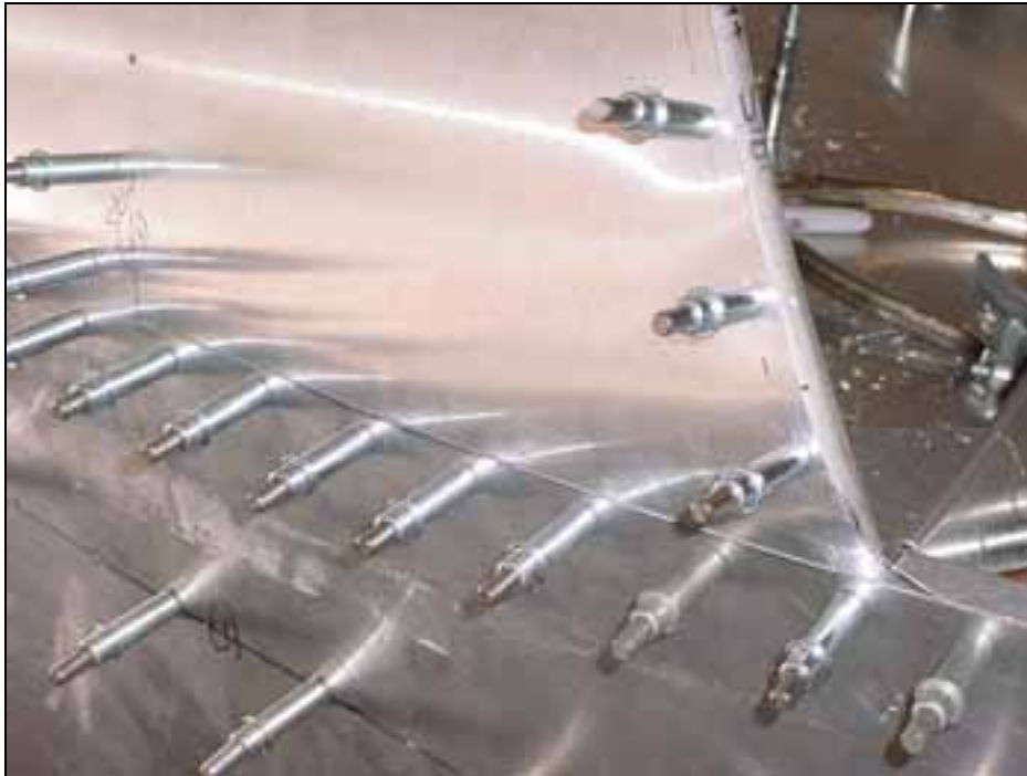
Overlap the side skin 6B11-2 on top of the middle top skin 6B21-7
