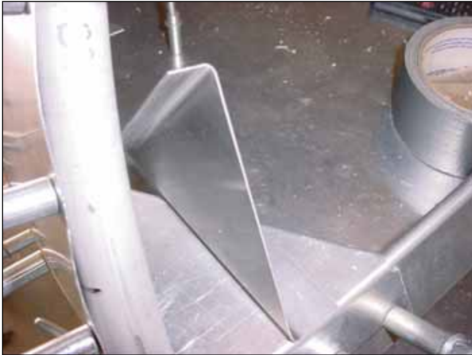
Top flange before it is trimmed.
