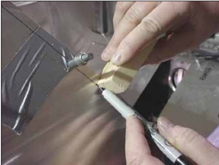
Marking the rivet line using the plywood template (front edge of 6B21-7)
