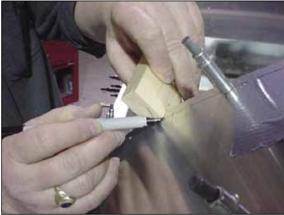
Marking the rivet line along the front edge of the Middle Top Skin 6B21-7 through the middle of the Tube Frame 6B21-1.
