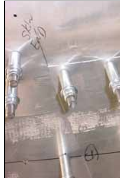
Compound curve: The rear just behind the side skins is where the top skin tends to bulge out.
