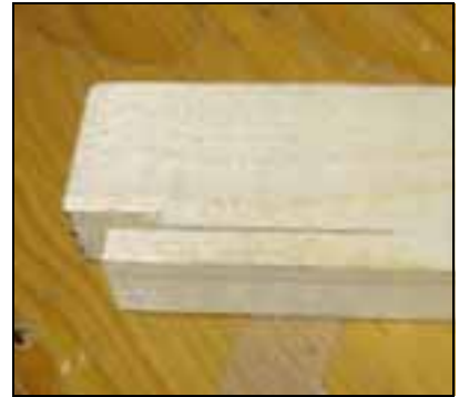
Marking template: wood block with a slot (the skin rides inside the slot), to mark the center of the top on the topside of the skin.
