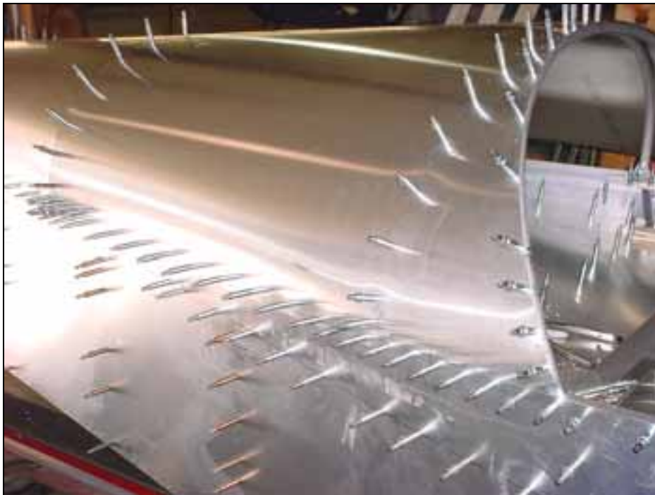
Layout the rivet line through the longeron 6B11-1
