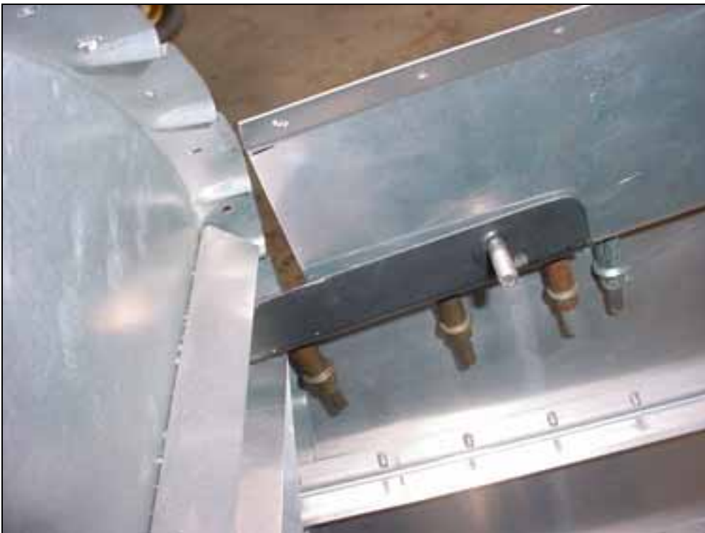
Corner would otherwise interfere with rubber trim when canopy is in the open position.
