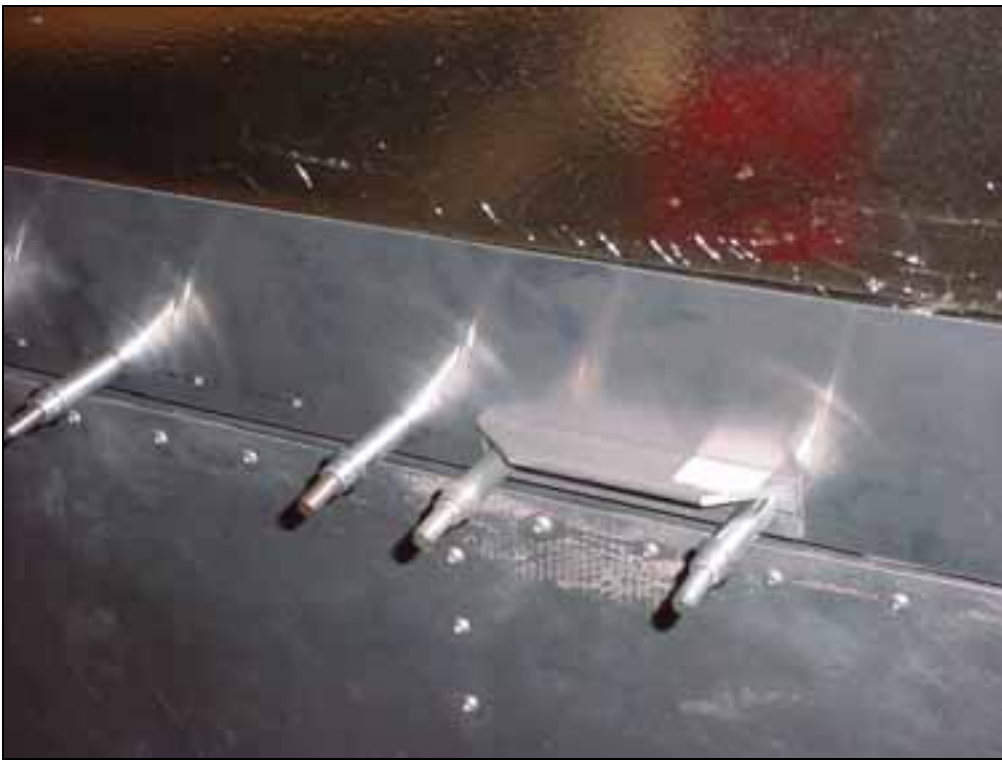
Extrusion handle 6C3-8 positioned in line with the latch. Ref. top right diagram on drawing 6-C-3
