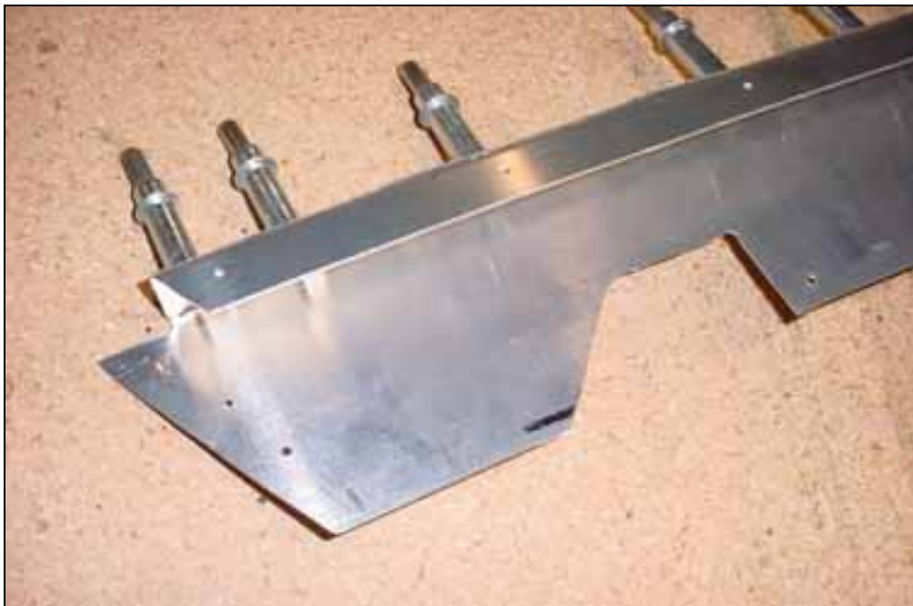
Inside Angle 6C3-4 clecoed to the inside flashing 6C3-5
