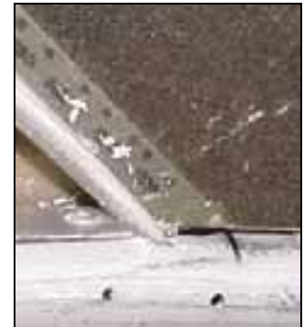
With a file open the hole along the bottom and top (elongated hole for cable housing)
