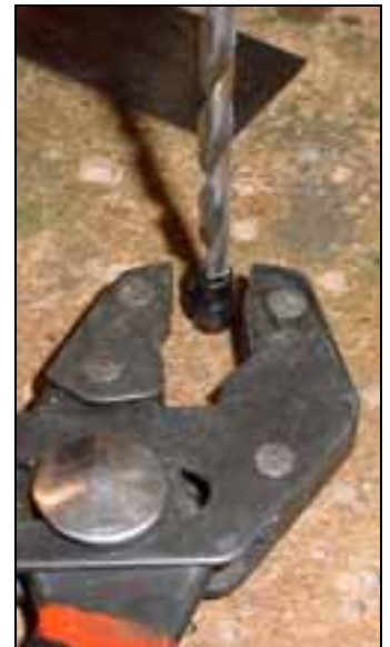
Run a drill bit through the plastic sleeve to fit over the cable housing.
