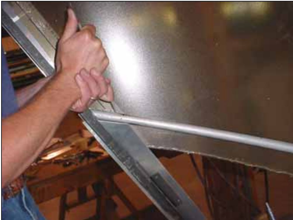
Drill a 3/16" in the front tube 6C3-2 just above the gusset 6C3-9
