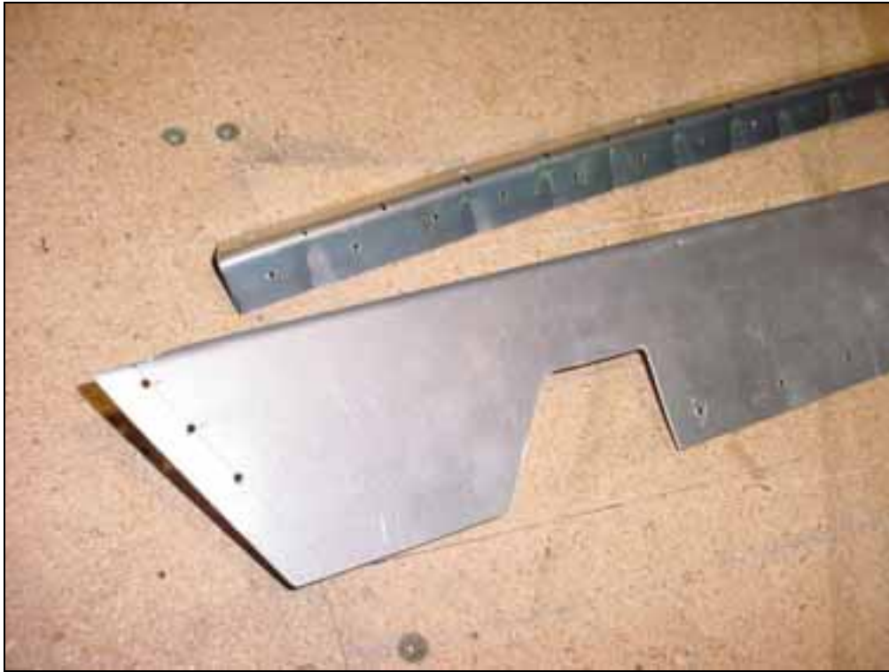
3 rivets A4 inside flashing to the 7/8" tube welded on the canopy frame.
