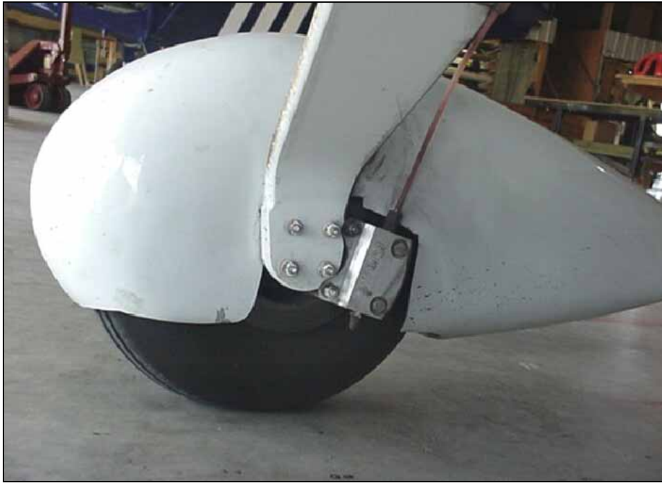
Right wheel File notches in gear to make room for calipers. Above photo shows gear installed opposite of recommended direction.
