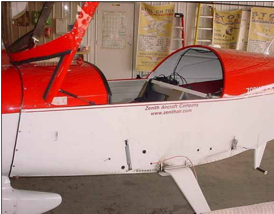
Brake line grommet in side of fuselage, behind spar and in front of the Front seat panel 6B15-4. Above photo shows gear installed opposite of recommended direction.
