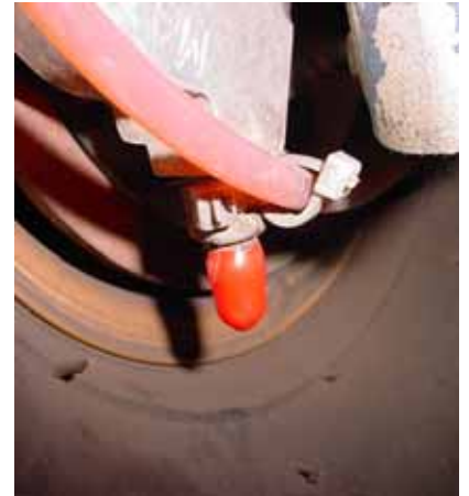
location of bleed screw at the bottom of the caliper (on one each wheel).
