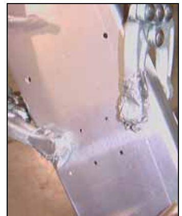
Clamp the rib to the spar. Use the toggle clamps.
