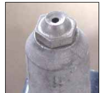
Special machined riveter nose piece
