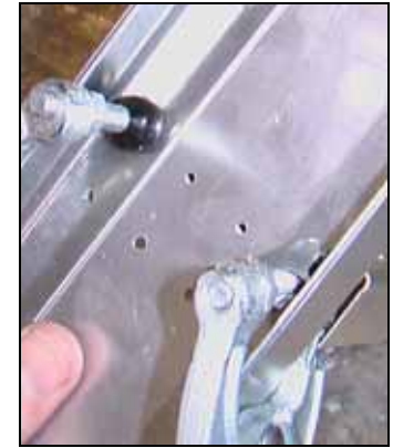
Clamp the rib to the spar.
