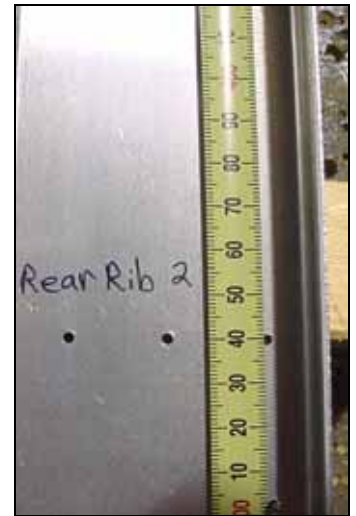
The pre-drilled holes in the spar web are measured from the bottom end of the doublers. Refer to drawing 6-T-5 for the rib locations.
