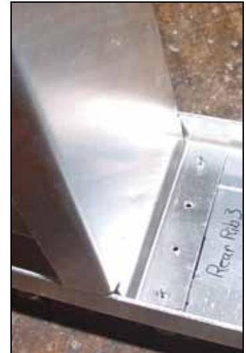
Rear rib #3, the spar flange points down, the side flanges point up.
