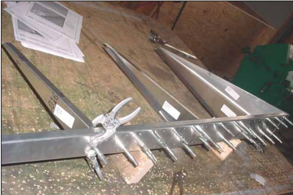
Rear rib #3, the spar flange points down, the side flanges point up.
