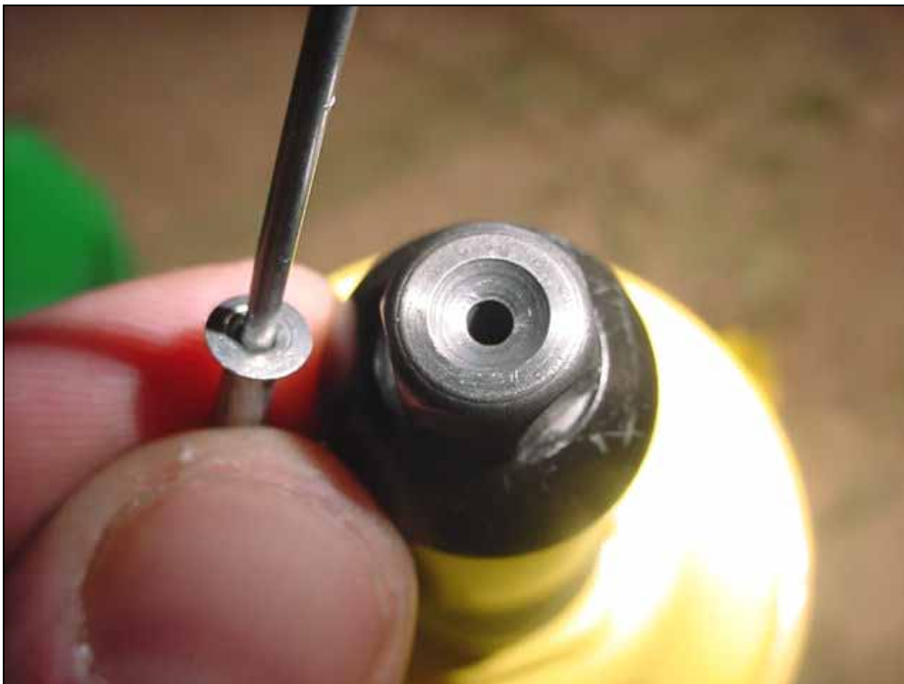
Special machined riveter nose piece
