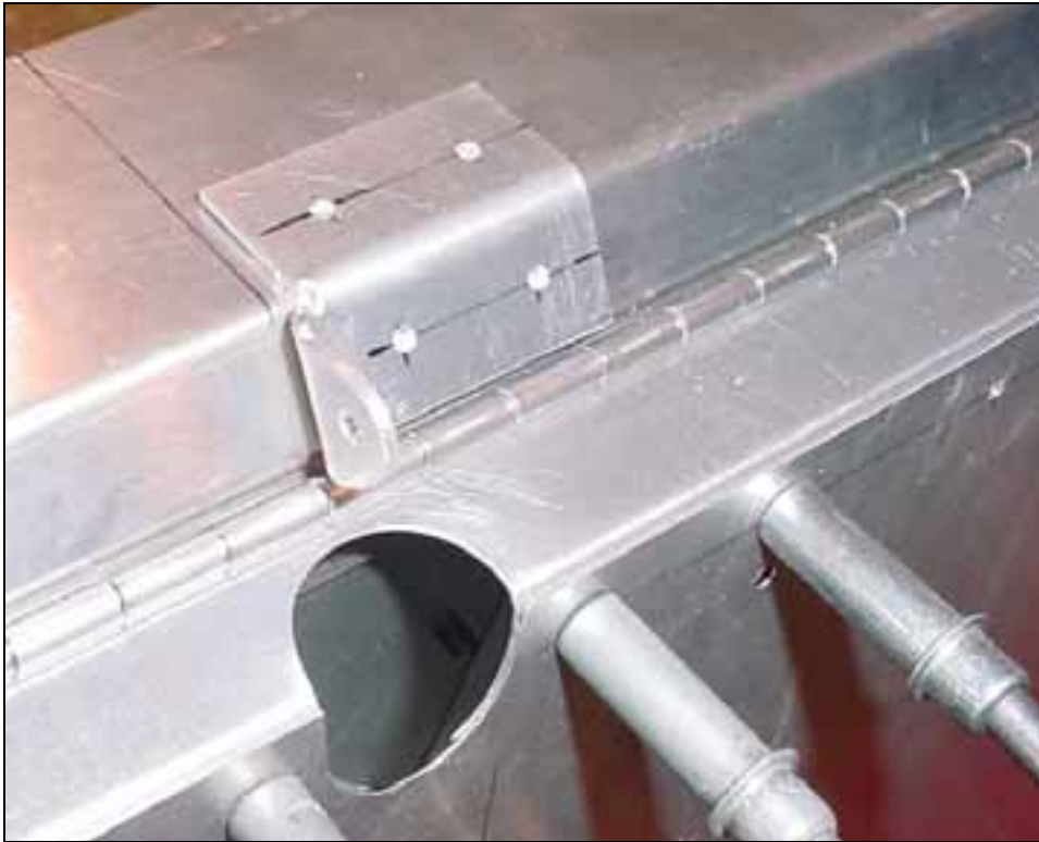
The Horn is positioned on the I/B side of the trim tab centerline.
