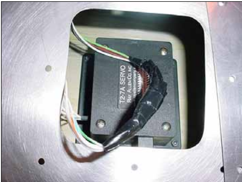
4 RIVETS A4 Servo to skin (rivets pulled from top side of the skin).
