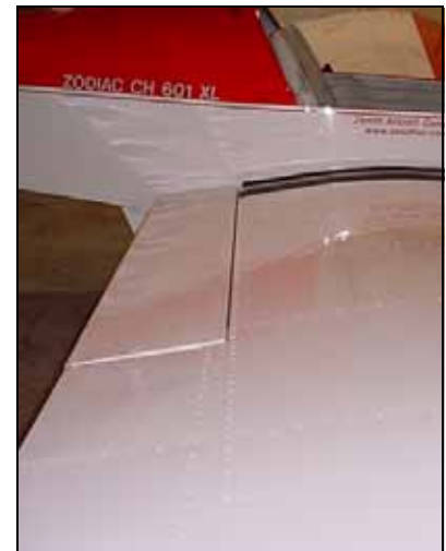
Note: the first flap rib does not line up with the rear ribs.
