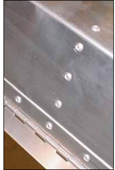
Rivet at the intersection of the rib station with the rivet line through the piano hinge.
