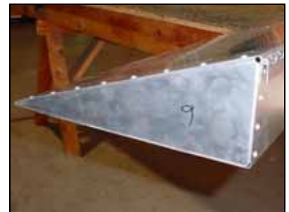
CHECK: There is no gap between the top skin and the rib.
