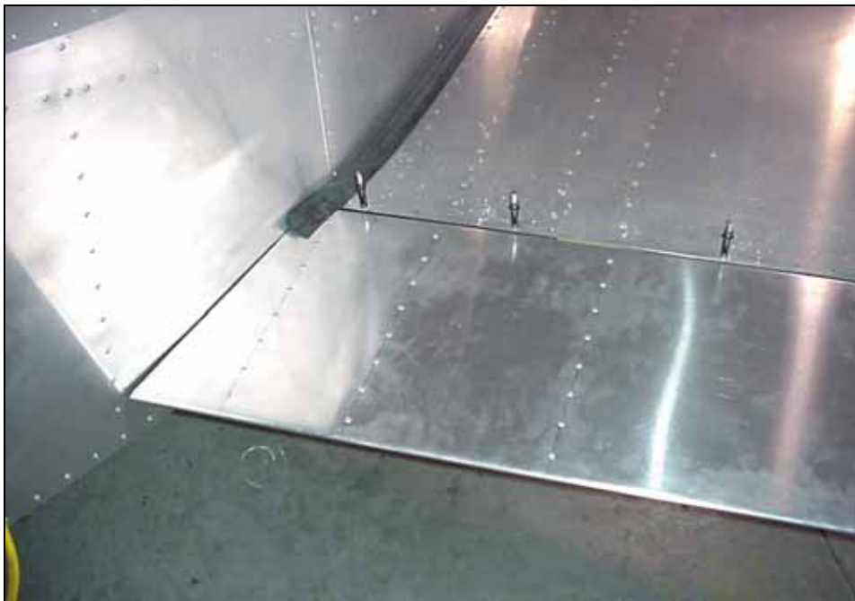
Note: the first flap rib does not line up with the rear ribs.
