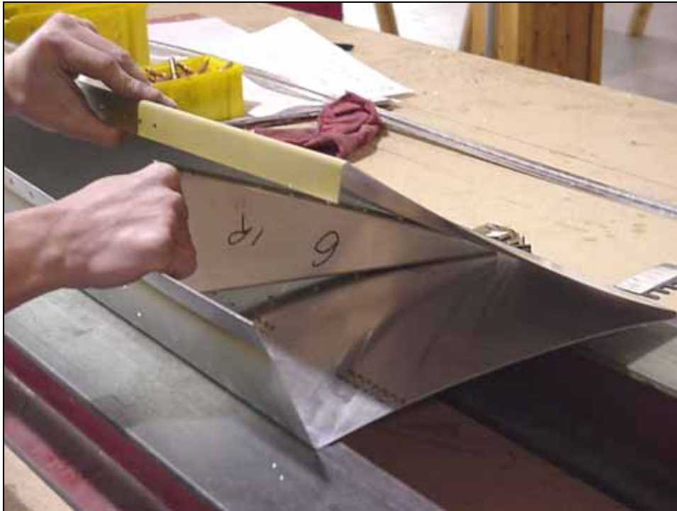
Position the ribs inside the flap skin.
