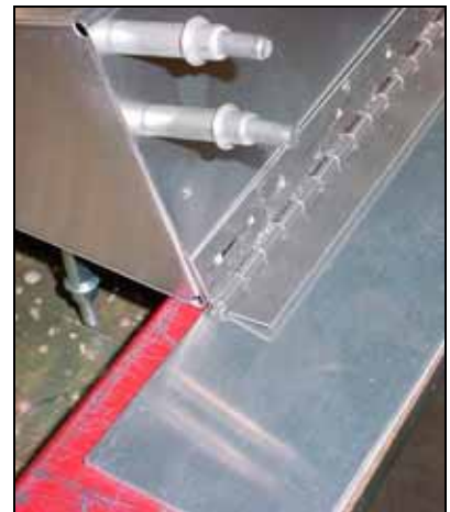
3mm offset from the bottom of the hinge to the bottom of the skin.
