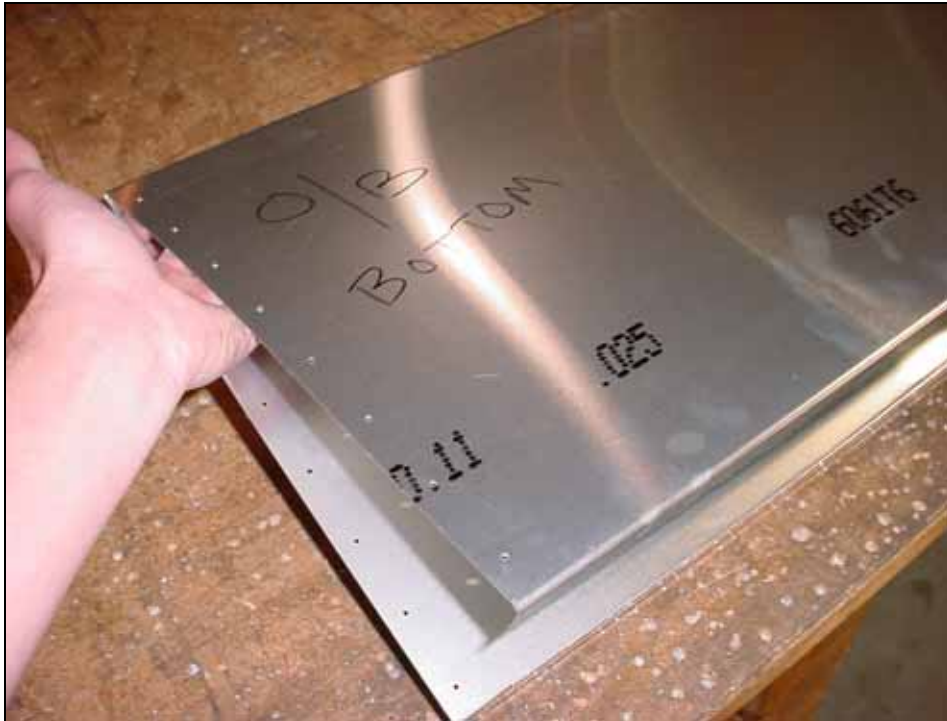
Pre-drilled holes in the skin.
