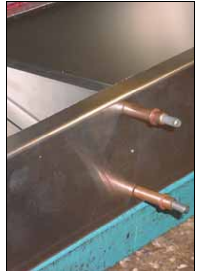
First drill and cleco 2 holes in each rib (front)
