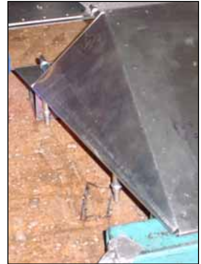
Turn the aileron over. Reposition the spacer block under the inboard trailing edge.
