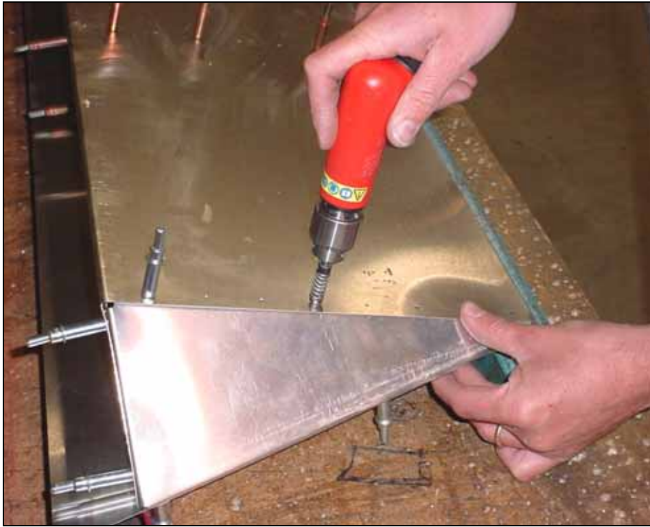
Drill and Cleco the bottom side of the tip rib.
