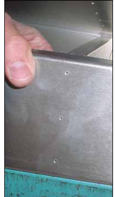
Line up the rib flange rivet line over the pre-drilled holes in the front of the aileron skin.
