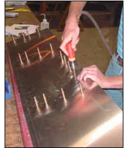
Drill the front flange.
