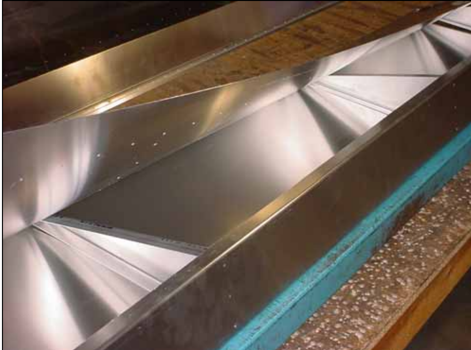
Position the middle ribs 6W2-2 (R) with the flange facing outboard.
