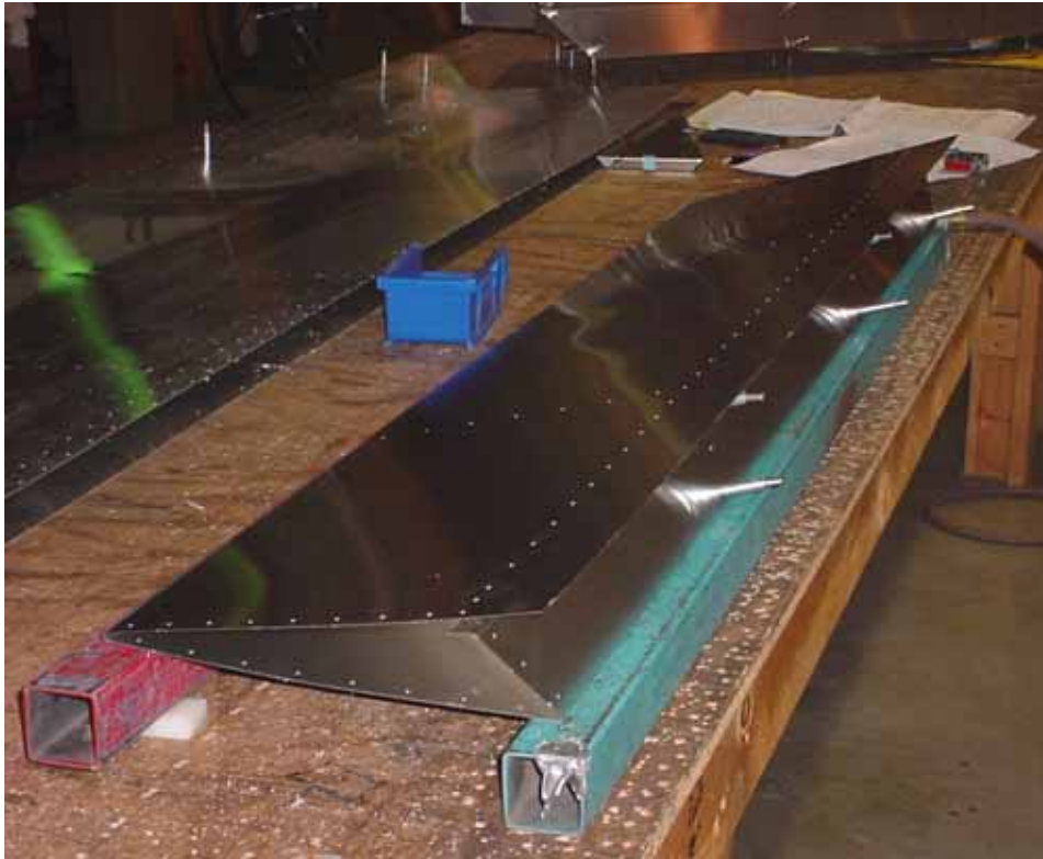
First drill and cleco 2 holes in each rib (front)
