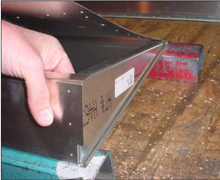
Install the I/B rib 6W2-3 (R) on the line.
