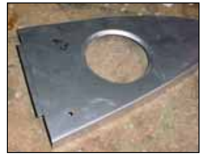
Nose Ribs 1, 2 and 3 See 6-W-7 for flange directions.
