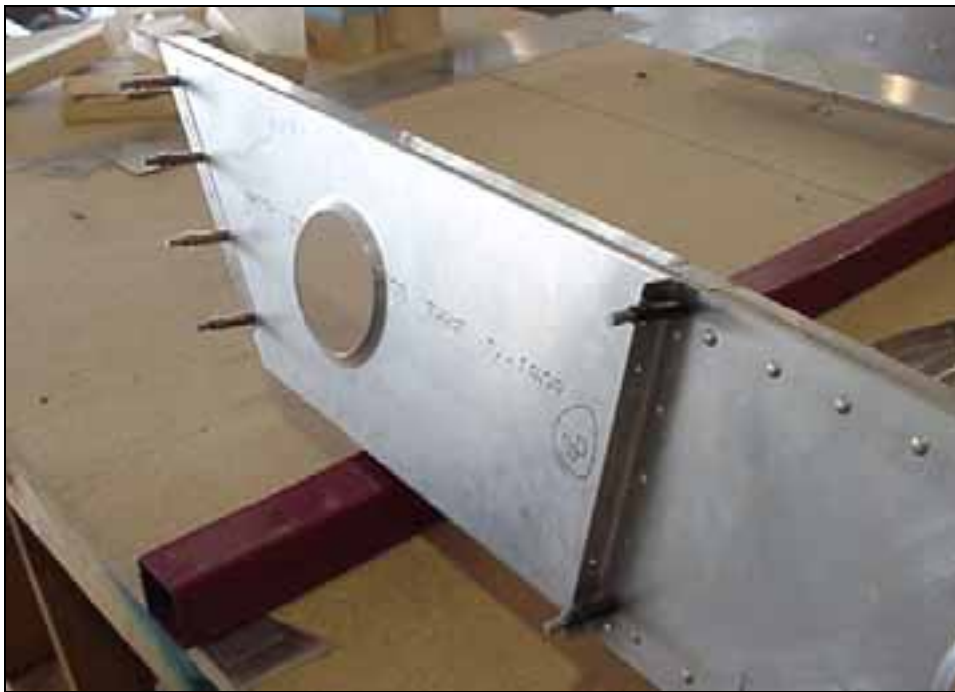
Looking at the front side of the spar assembly.
