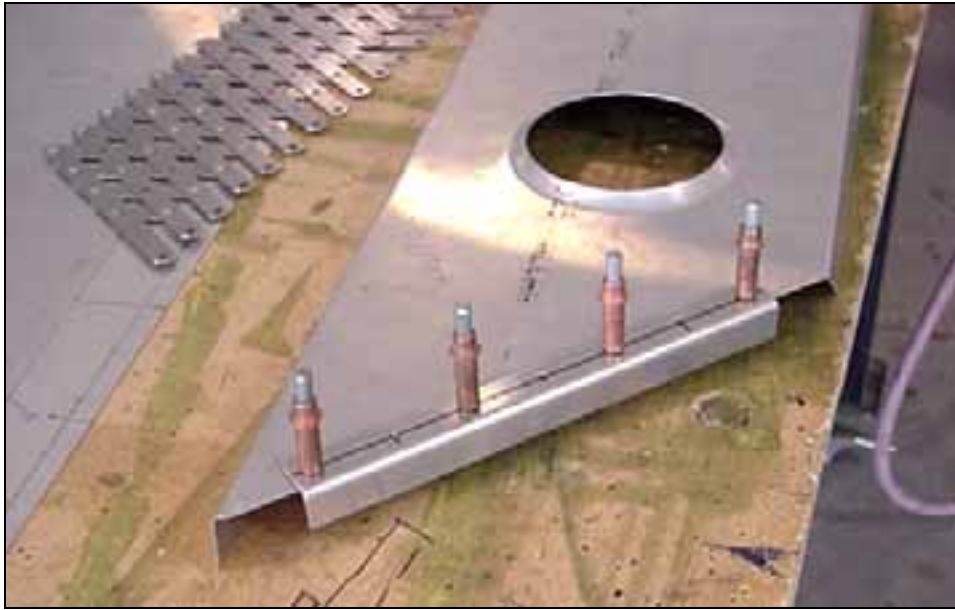
L angle clecoed to spar tip.
