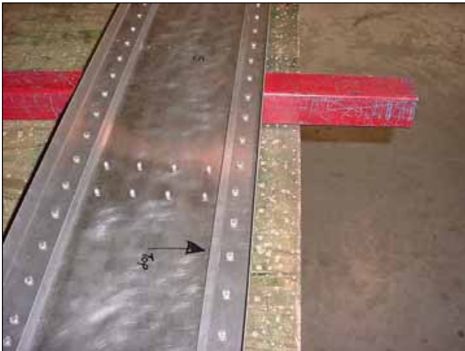
MARK: Identify the top side of the spar, and mark an arrow TOP (top spar cap angle 6W3-6 has the flange bend 90 degrees).
