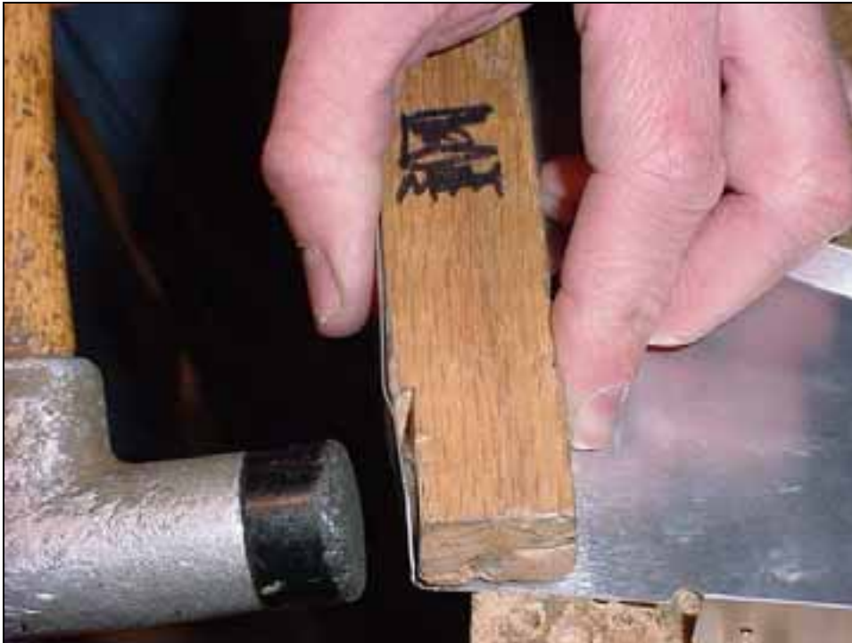
Joggling block: 3mm step by 25mm long
