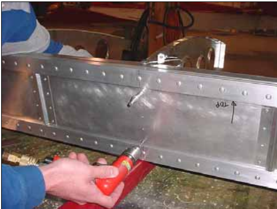
All the rear ribs are square to the top flange of the spar.
