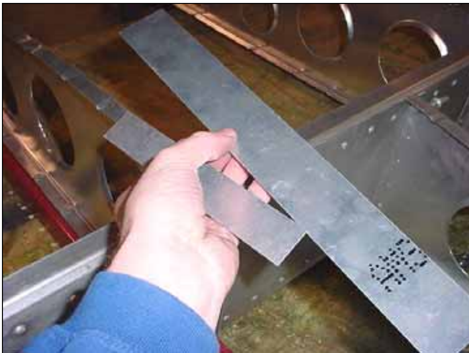
.025" strip top flange of cap angle 6W3-8
