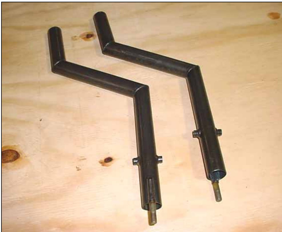
6DS3-1 CONTROL COLUMN
