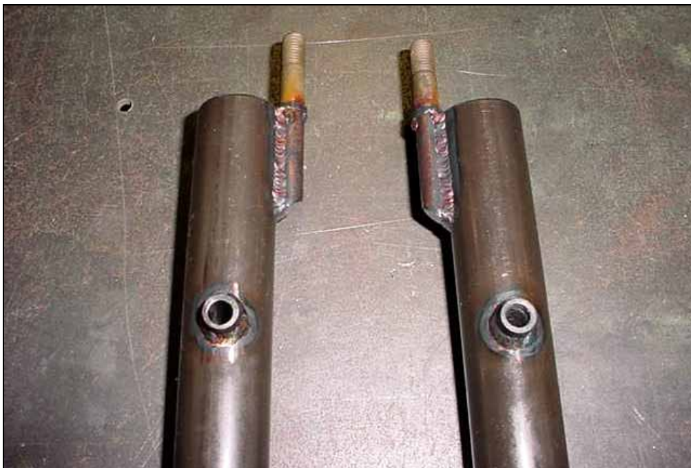
ORIENTATION: Position the control column over the edge of the workbench with the welded bolt on the I/B side.
