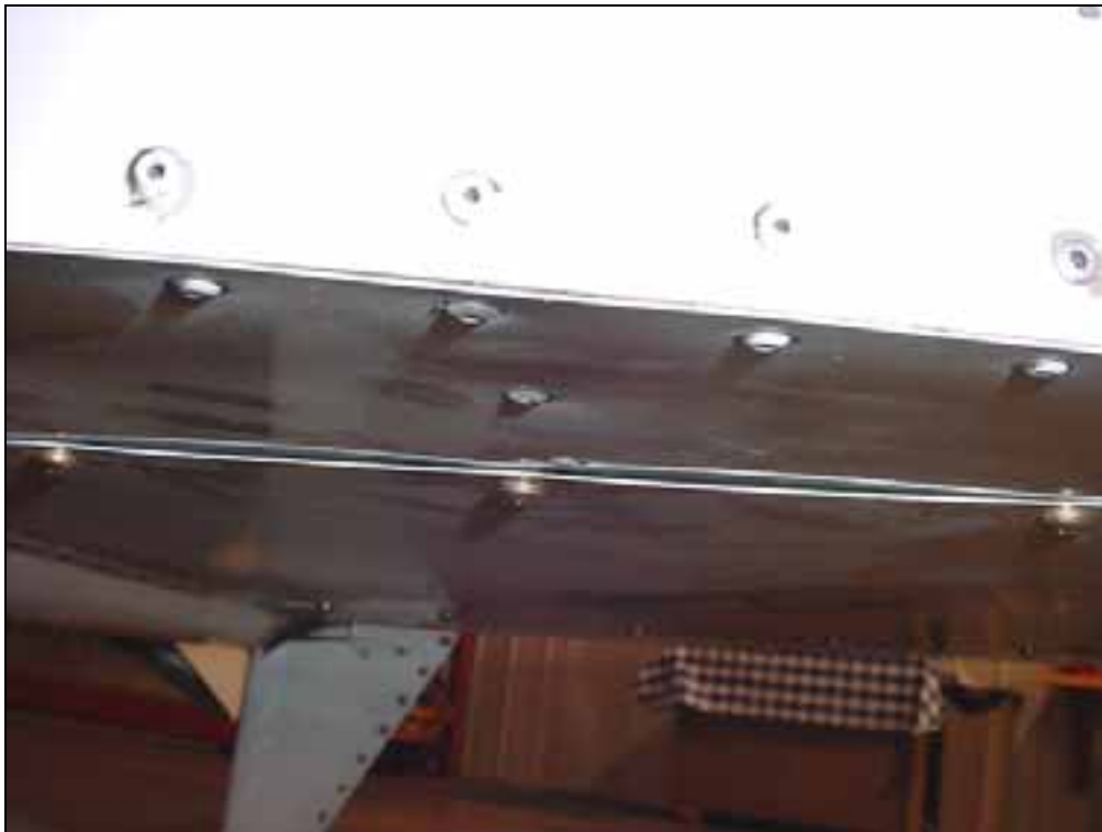
AN960-10 washer under screw.
