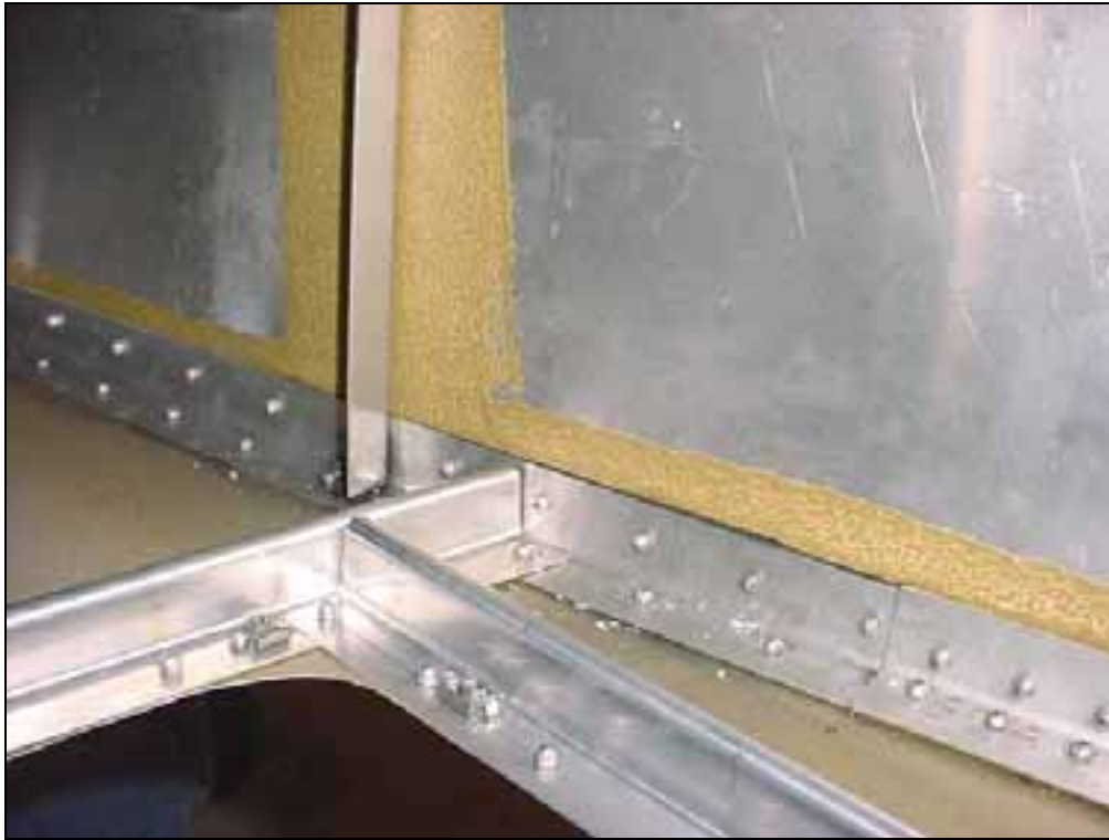
Z angle overlap on top of the Longeron 6B2-1
