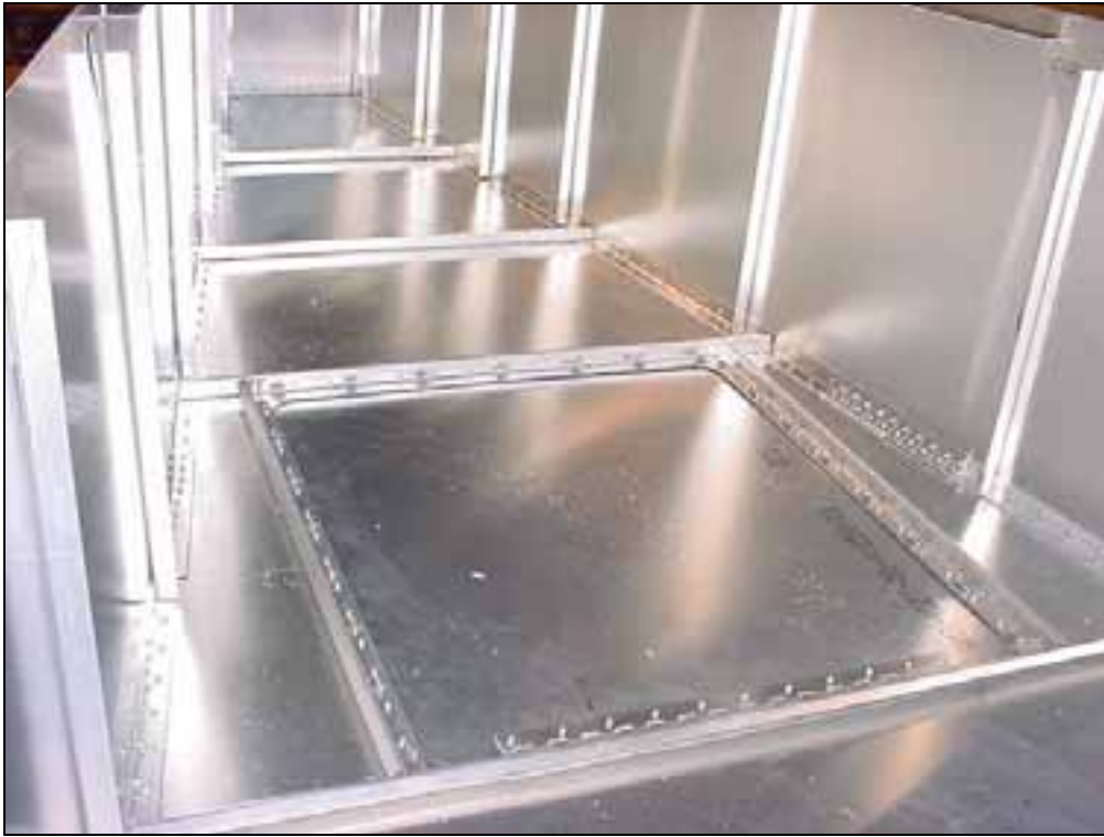
Looking inside the rear fuselage at the access door.
