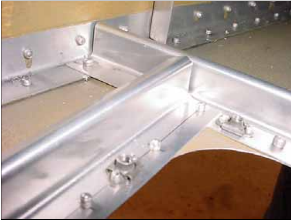
Rear right cutout Flanges overlap up to the bend tangent line of the bend.
