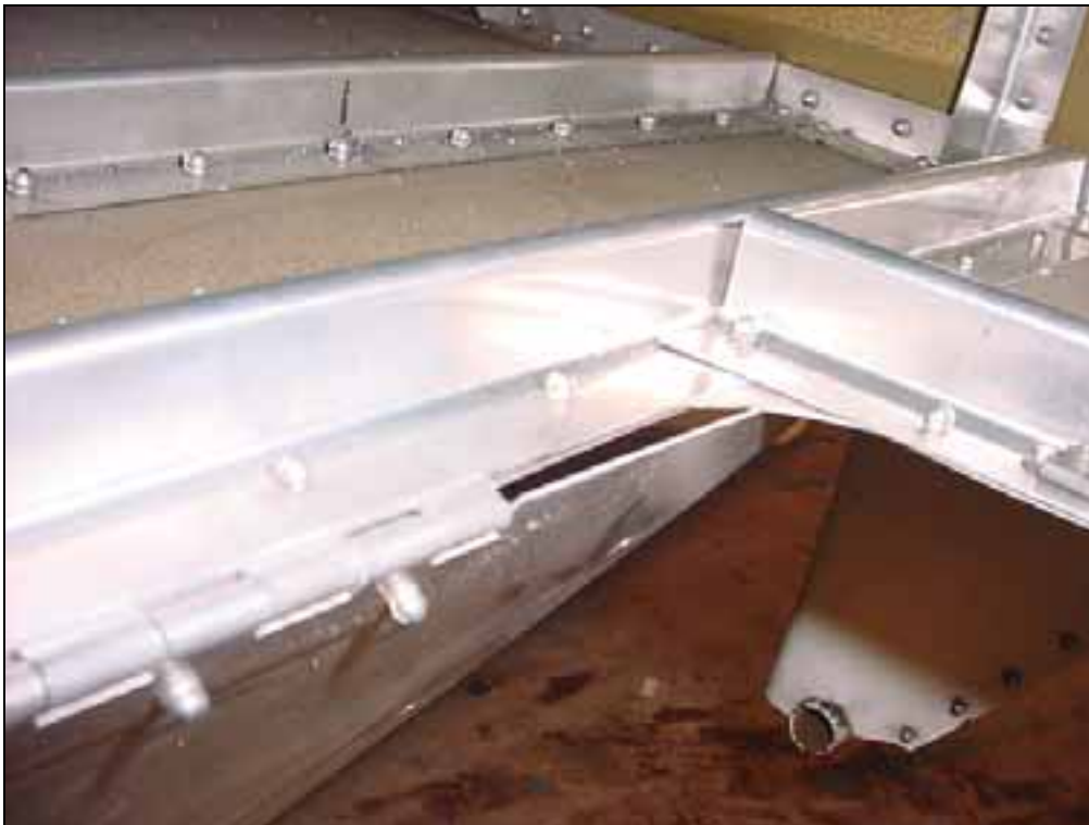
Cutout is framed with Z angles all around.
