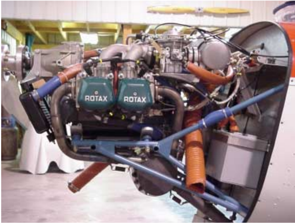
Battery on firewall
