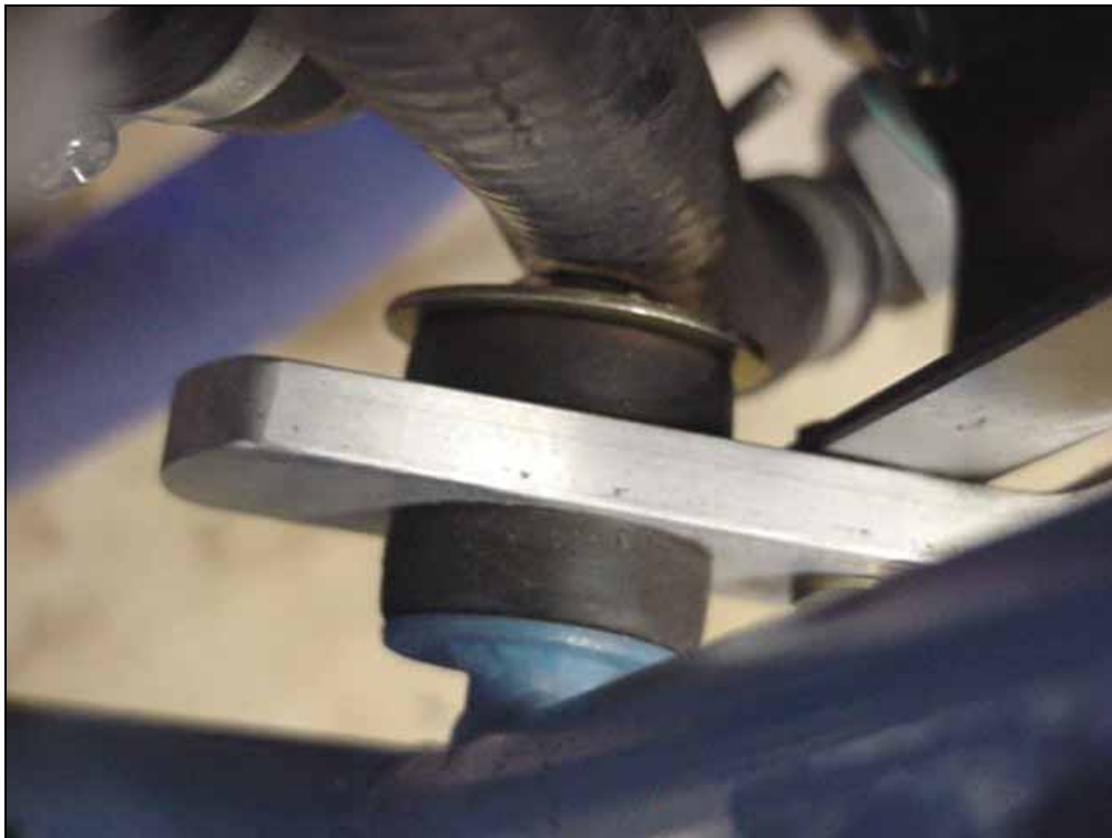
Rear right hose makes overtop the bolt
