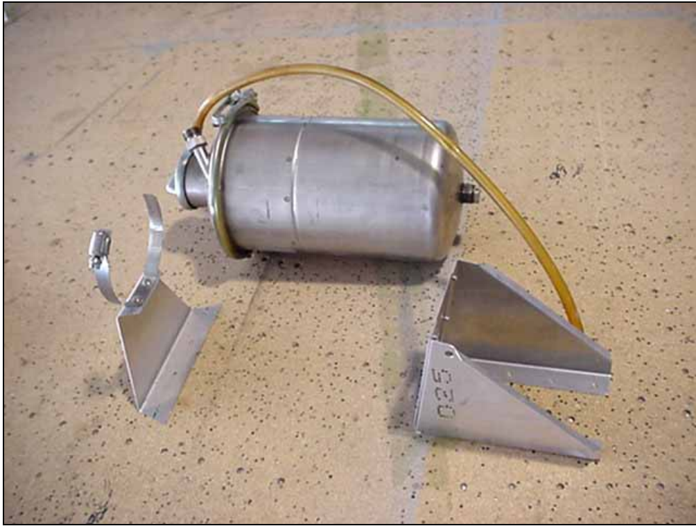
Oil reservoir for Rotax dry sump.
