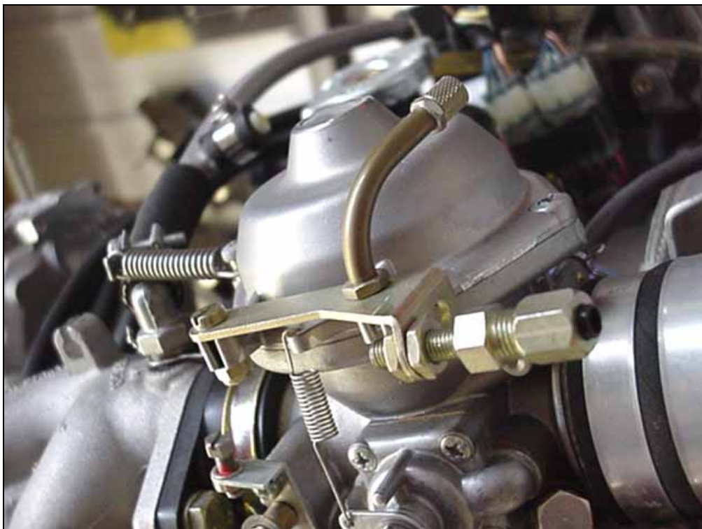
Remove the cable adjuster on the carburetor, open the hole in the mounting bracket and crew in the cable stop adjuster 25-0700
