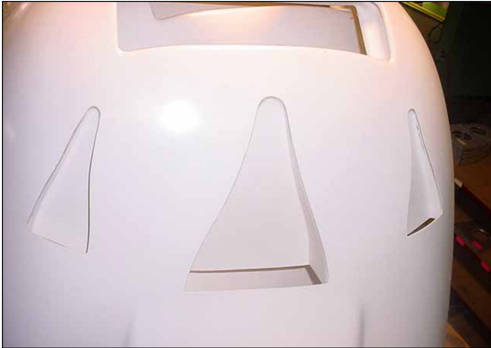
Outside view of NACA scoop for the oil cooler,
