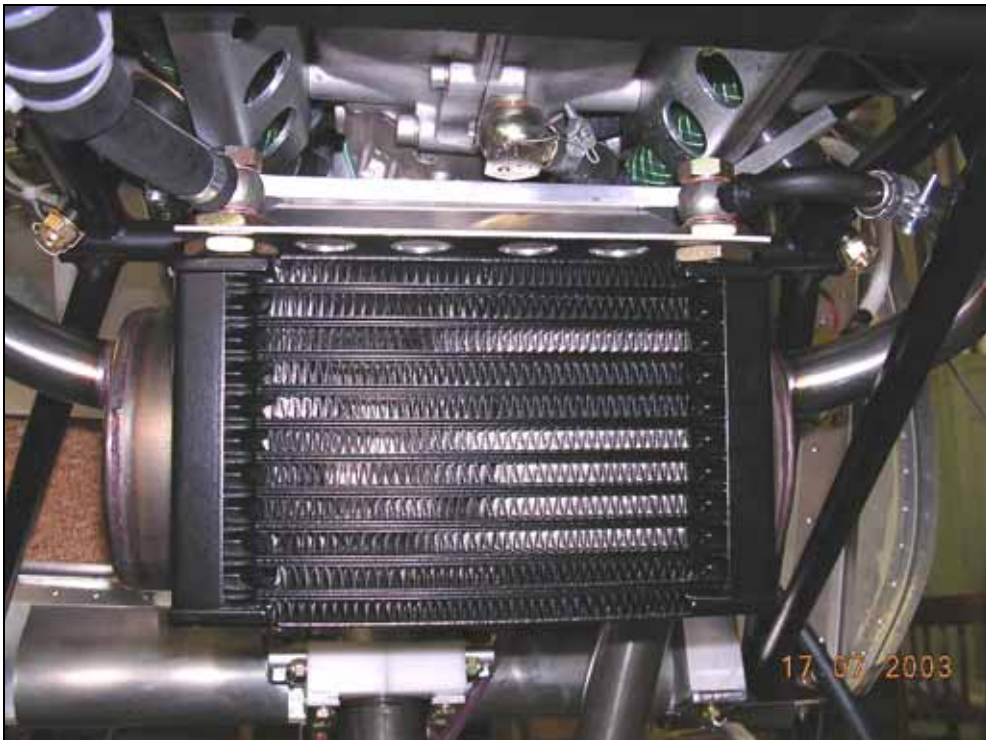
Oil cooler bracket bolted to rear Dynafocal Bracket E2-1X
