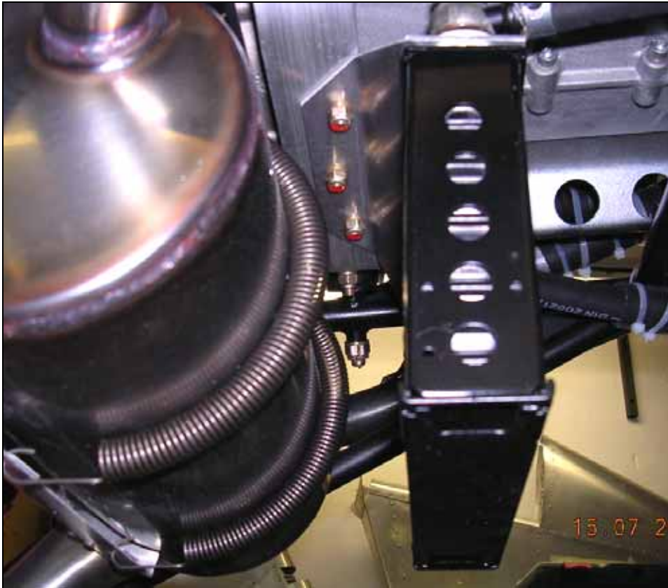
Oil cooler bracket bolted to rear Dynafocal Bracket E2-1X
