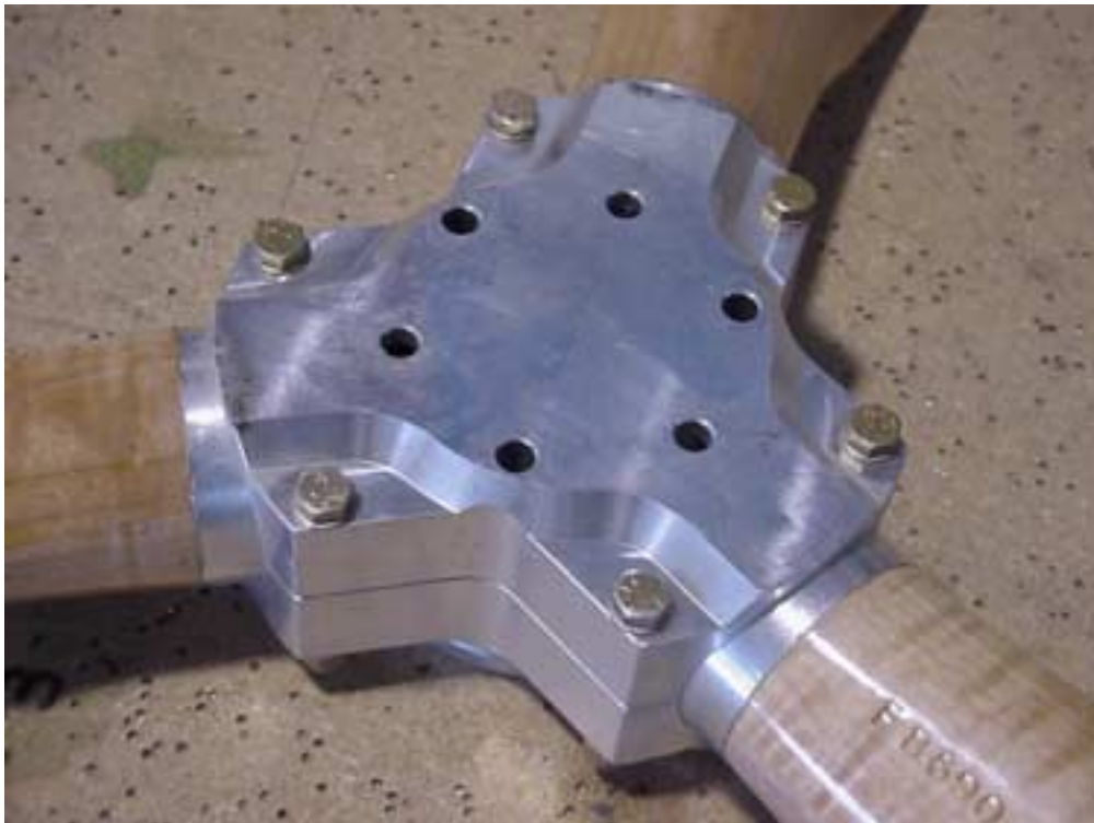
GSC wood prop with aluminum root ends
